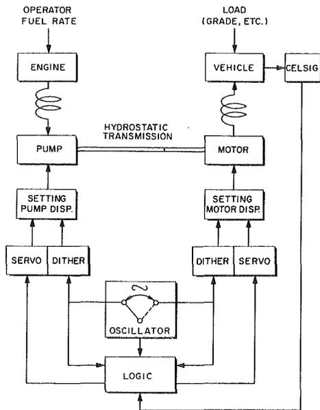
Fig. 13 Closed loop optimizer control for hydrostatic transmission
