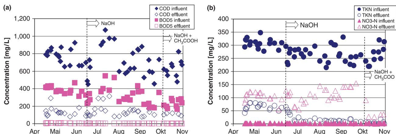
Figure 2 | COD and BOD<sub>5</sub> profiles (a) and TKN and NO<sub>3</sub>-N profiles (b) during operation.
