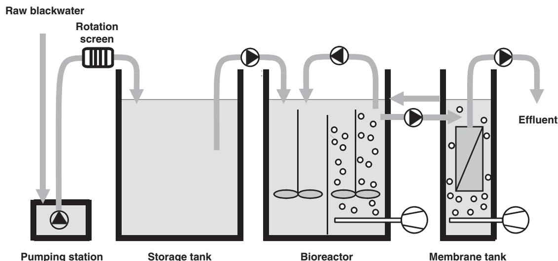
Figure 1 | Schematic layout of blackwater pilot plant.
