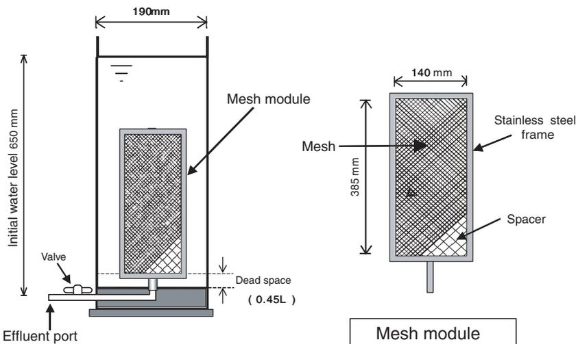
**Figure 1** Sludge thickening apparatus and filter module
