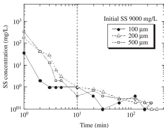
**Figure 3** Relationship between effluent SS and filtration period
