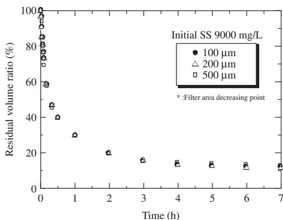
**Figure 2** Relationship between residual volume ratio and filtration period
