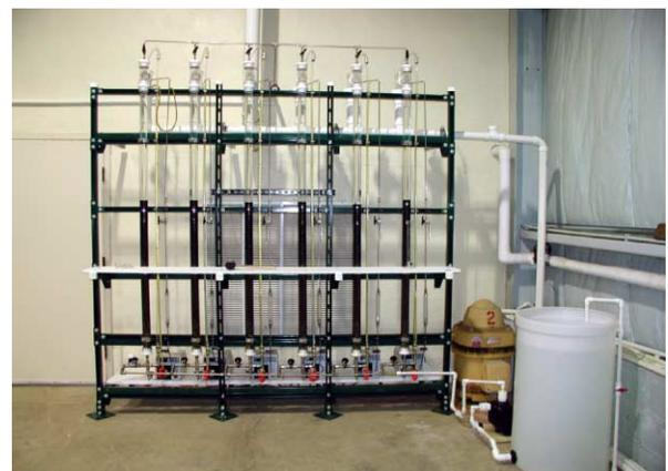
**Figure 4** | Photograph of pilot scale filtration system.
