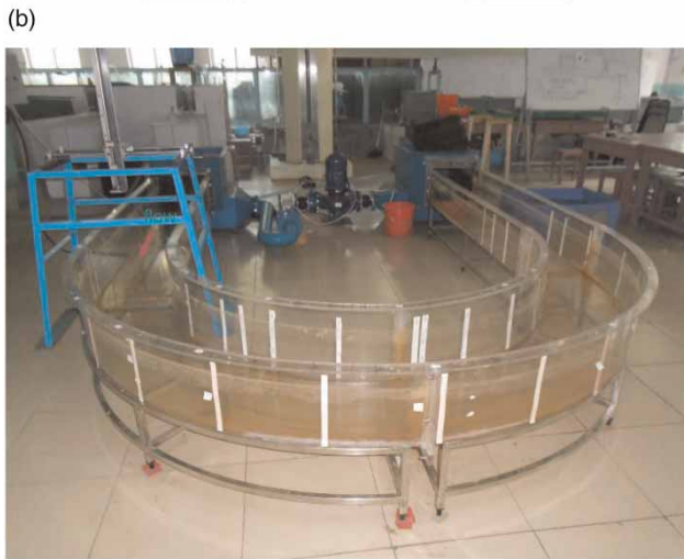
Figure 1 | (a) Schematic view of 180° channel and (b) picture of experimental set up.
