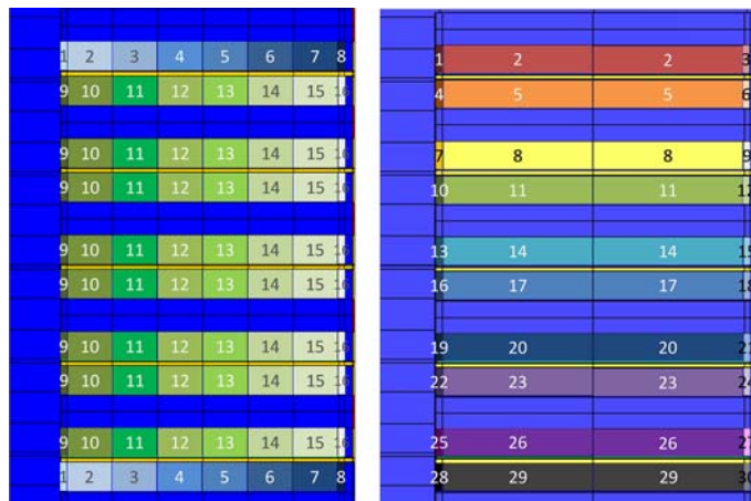
FIG. 7. Variant case arrangements of sub-models. Access tunnels are shown in yellow and reside in the whole repository model.
