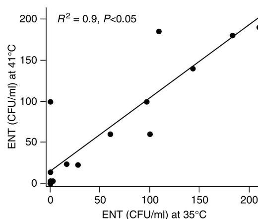
**Figure 2** | Comparison of two incubation temperatures (35°C and 41°C) for determining concentrations of enterococci in water samples. Identical volumes of the same water sample were filtered, placed on mEI agar, and incubated either at 35°C (x-axis) or 41°C (y-axis). Line shows least-squares regression.
