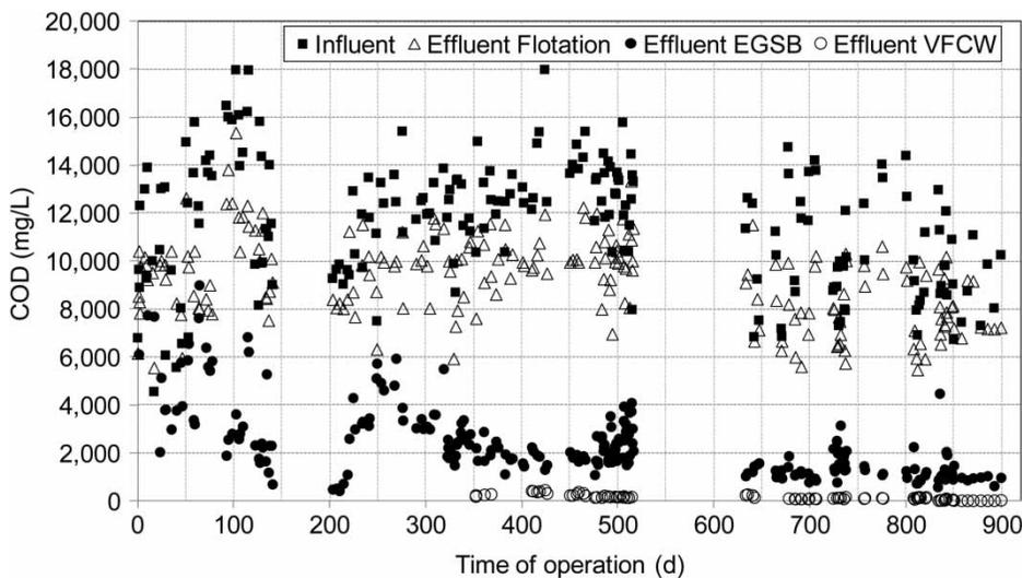
Figure 2 | Influent and effluent COD concentrations during 2.25 years of operation.
