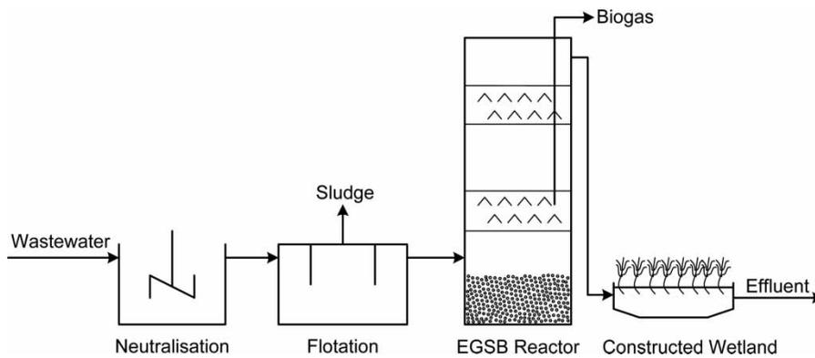
Figure 1 | Scheme of the treatment concept.
