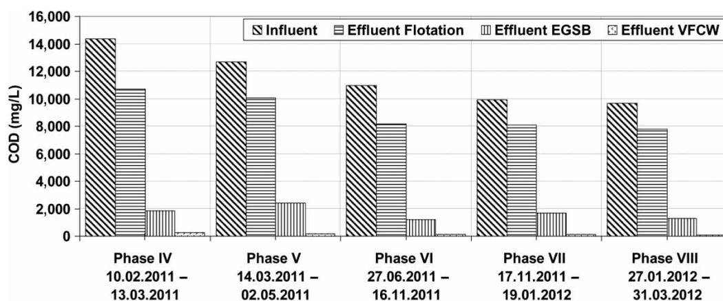
Figure 3 | Mean COD concentrations during the last five operating phases.
