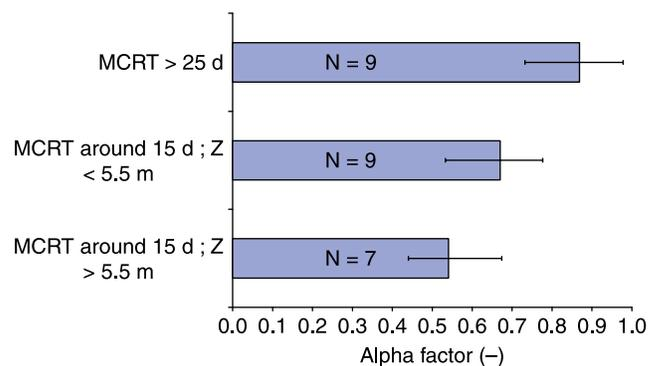
Figure 3 | Alpha factor for different MCRT and diffuser submergences (| - | extreme values).
