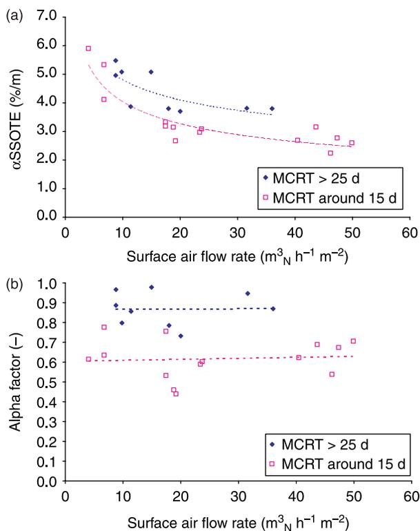
Figure 2 |  $\alpha$ SSOTE (2a) and alpha factor (2b) versus surface air flow rate.
