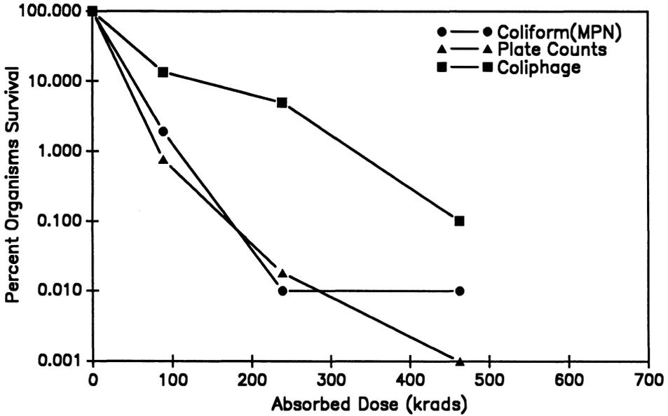
Fig.1. Disinfection of Raw Wastewater with Gamma Irradiation
