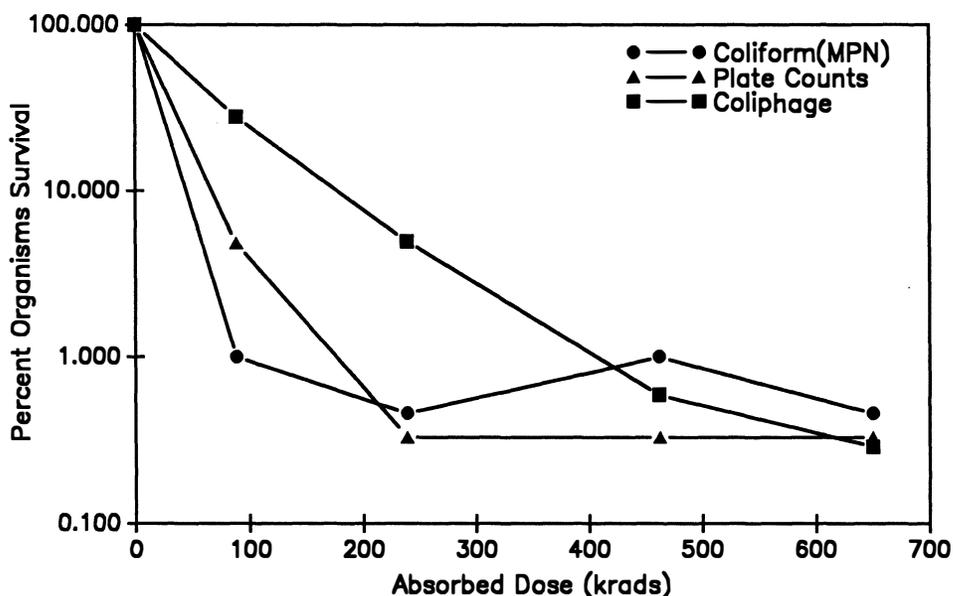
Fig.3. Disinfection of Raw Wastewater with E-Beam
