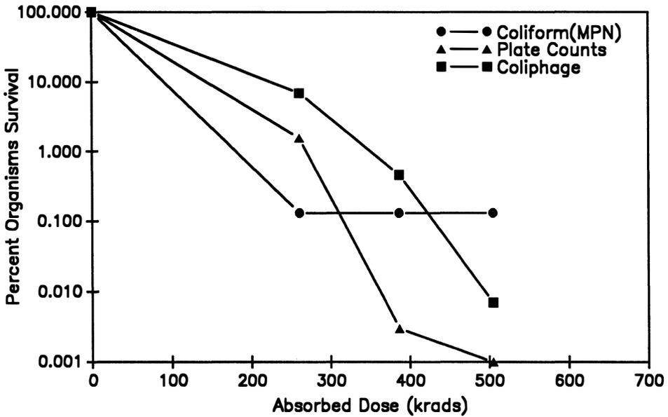
Fig.2. Disinfection of Secondary Effluent with Gamma Irradiation
