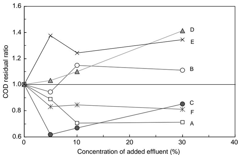
**Figure 5** Relationship between concentration of added effluent and COD Residual ratio
