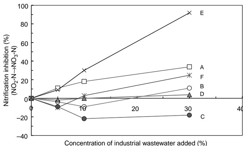
Figure 3 Concentration of industrial wastewater added and nitrification inhibition
