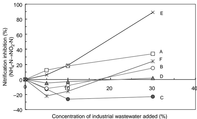
**Figure 4** Concentration of industrial wastewater added and nitrification inhibition
