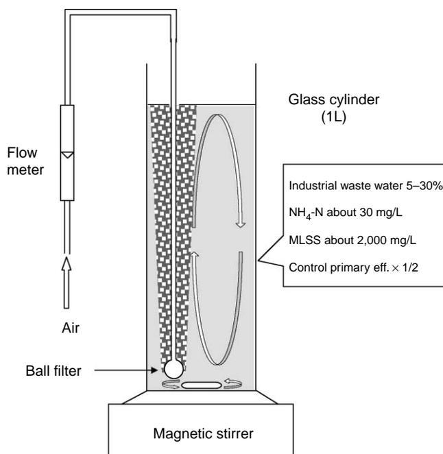
**Figure 2** The test equipment for nitrification inhibition
