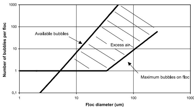
**Figure 10** | Number of available and attachable bubbles for every floc as a function of floc diameter (conditions:  $C_f=5 \text{ mg l}^{-1}$ ,  $C_b=8 \text{ mg l}^{-1}$ ,  $d_b=60 \text{ }\mu\text{m}$ ,  $D_{fr}=2.2$ ).
