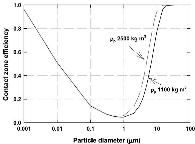
**Figure 3** | Effect of the particle or floc density ( $\rho_p$ ) on the contact zone efficiency as a function of particle or floc size (conditions:  $t_{cz}=3$  min,  $T=293$  K,  $a_{pb}=0.5$ ,  $d_b=60$   $\mu\text{m}$ , and  $\phi_b=8,000$  ppm).
