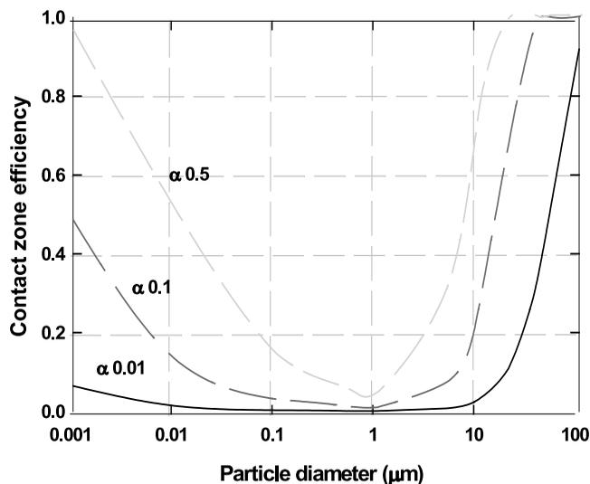
**Figure 2** | Effect of the particle–bubble attachment factor ( $\alpha_{pb}$ ) on the contact zone efficiency as a function of particle or floc size (conditions:  $t_{cz}=3$  min,  $T=293$  K,  $\rho_p=1,100$  kg m $^{-3}$ ,  $d_b=60$   $\mu$ m, and  $\phi_b=8,000$  ppm).
