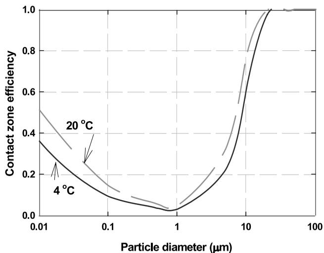
**Figure 4** | Effect of water temperature on the contact zone efficiency as a function of particle or floc size (conditions:  $t_{cz}=3$  min,  $a_{pb}=0.5$ ,  $\rho_p=1,100$   $\text{kg m}^{-3}$ ,  $d_b=60$   $\mu\text{m}$ , and  $\phi_b=8,000$  ppm).
