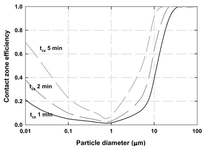
**Figure 7** | Effect of contact zone time on contact zone efficiency as function of particle or floc size (conditions:  $T=293\text{ K}$ ,  $a_{pb}=0.5$ ,  $\rho_p=1,100\text{ kg m}^{-3}$ ,  $d_b=60\text{ }\mu\text{m}$ , and  $\phi_b=8,000\text{ ppm}$ ).
