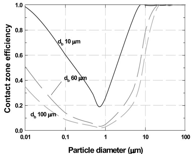
**Figure 5** | Effect of bubble diameter on contact zone efficiency as a function of particle or floc size (conditions:  $t_{cz}=3$  min,  $T=293$  K,  $a_{pb}=0.5$ ,  $\rho_p=1,100$   $\text{kg m}^{-3}$ , and  $\phi_b=8,000$  ppm).
