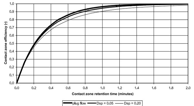
Figure 13 | Effect of axial dispersion on the contact zone efficiency (conditions:  $d_b=60 \mu\text{m}$ ,  $\mu_b=0.5$ ,  $d_f=30 \mu\text{m}$ ,  $\varphi_b=6,000 \text{ ppm}$ ,  $T=293 \text{ K}$ ,  $D_{sp}=0.05$  and  $0.2$ ).
