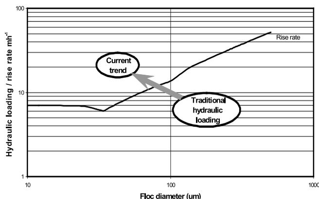
**Figure 14** | Evolution of DAF design parameters from the 1970s to the 1990s in comparison with theoretical floc-bubble rise rates presented in Figure 11.
