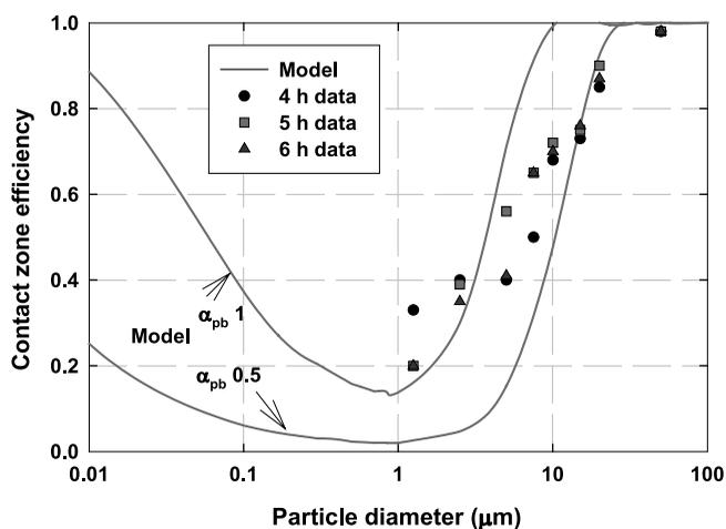
**Figure 8** | Model versus experimental data (model assumptions:  $d_b=60\ \mu\text{m}$  and  $\alpha_{pb}$  of 0.5 and 1; experimental conditions: DAF loading rate  $15\ \text{m h}^{-1}$ ,  $t_{cz}=1.9\ \text{min}$ ,  $T=278.5\ \text{K}$ ,  $\phi_b=7,840\ \text{ppm}$ ).
