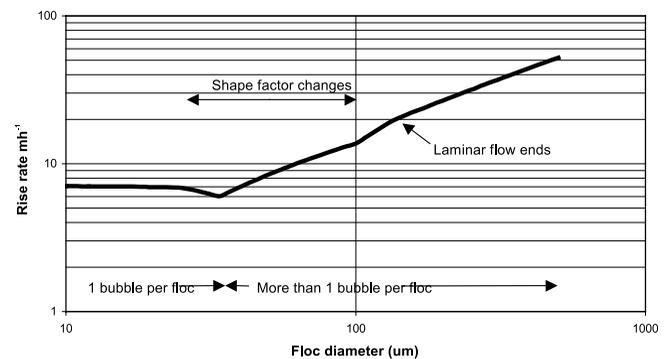
**Figure 11** | Calculated rise rate for floc–bubble aggregates grown from kaolin primary particles, assuming maximum air efficiency and the densest possible bubble packing (conditions:  $C_f=5 \text{ mg l}^{-1}$ ,  $d_b=60 \text{ }\mu\text{m}$ ,  $D_{fr}=2.2$ ,  $T=20^\circ\text{C}$ ).
