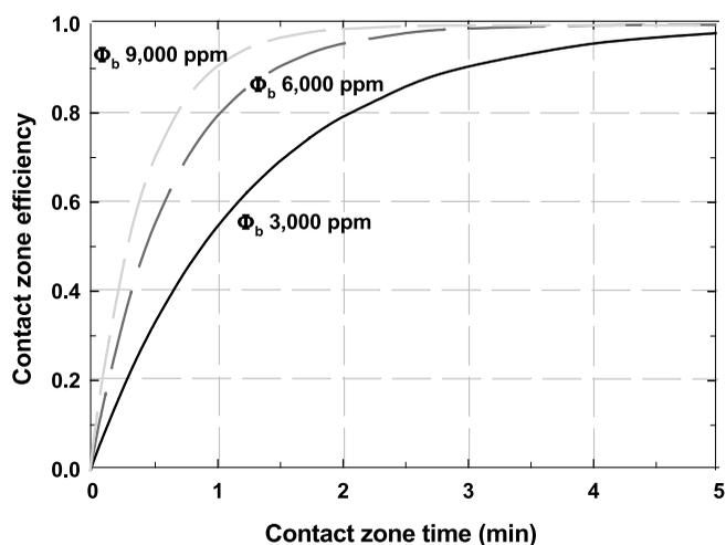
**Figure 6** | Effect of bubble volume concentration on the contact zone efficiency as a function of contact zone time for 20  $\mu\text{m}$  flocs (conditions:  $T=293\text{ K}$ ,  $a_{pb}=0.5$ ,  $\rho_p=1,100\text{ kg m}^{-3}$ , and  $d_b=60\text{ }\mu\text{m}$ ).
