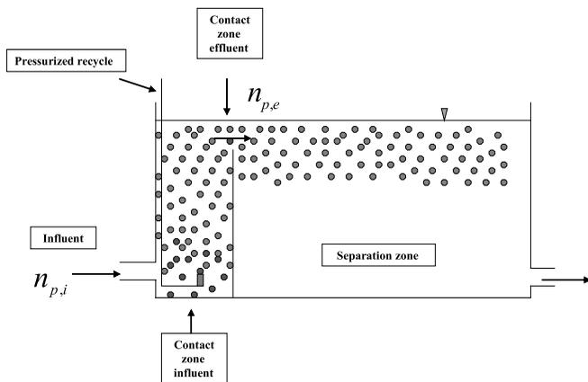
**Figure 1** | Schematic of a DAF tank showing a blanket of air bubbles in the baffled section of the contact zone extending into the top part of the separation zone.
