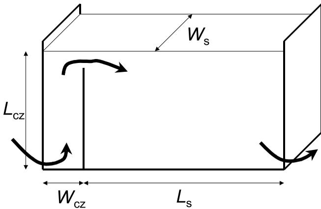
Figure 12 | Assignment of length L and width W to the contact and separation zones.
