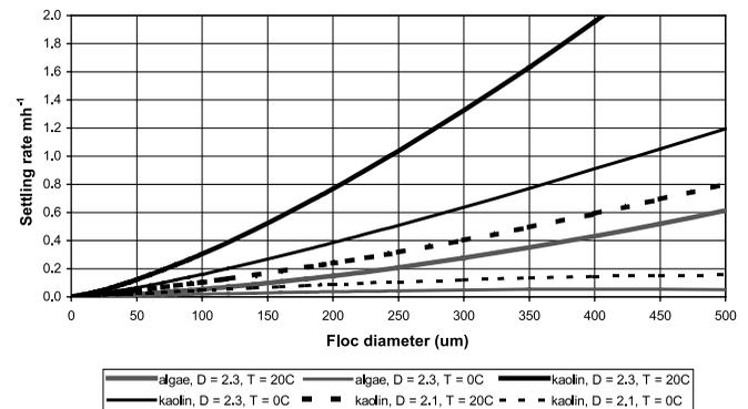
**Figure 9** | Calculated floc settling rates for different suspension types, temperatures and fractal dimensions (conditions for kaolin:  $d_p=0.3 \mu\text{m}$ ,  $\rho_p=2,650 \text{ kg m}^{-3}$ ; conditions for algae:  $d_p=10 \mu\text{m}$ ,  $\rho_p=1,020 \text{ kg m}^{-3}$ ).
