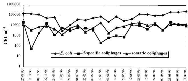
**Figure 8a** | Concentrations of *E. coli*, somatic and f-specific coliphages ( $\log cfu ml^{-1}$ ) in primary treated sewage, results for the plant at HG.
