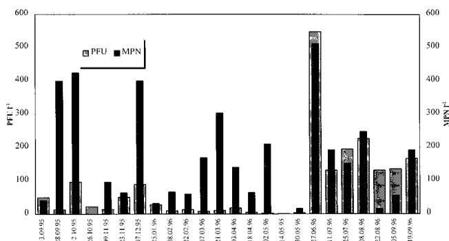
**Figure 5a** | Concentrations of viruses in primary treated sewage ( $l^{-1}$ ), results for the plant at WE. The results given as PFU show concentrations of enteroviruses enumerated as plaque-forming-units, results given as MPN show concentrations of other enteric viruses enumerated as most probable number.
