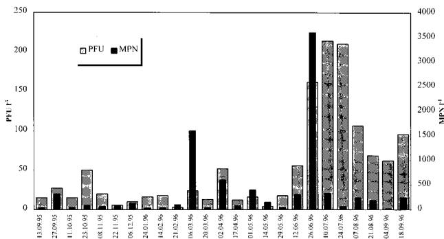
**Figure 7a** | Concentrations of viruses in primary treated sewage ( $l^{-1}$ ), results for the plant at HG. The results given as PFU show concentrations of enteroviruses enumerated as plaque-forming-units, results given as MPN show concentrations of other enteric viruses enumerated as most probable number.
