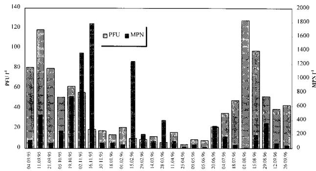
**Figure 3a** | Concentrations of viruses in primary treated sewage ( $l^{-1}$ ), results for the plant at RT. The results given as PFU show concentrations of enteroviruses enumerated as plaque-forming-units, results given as MPN show concentrations of other enteric viruses enumerated as most probable number.
