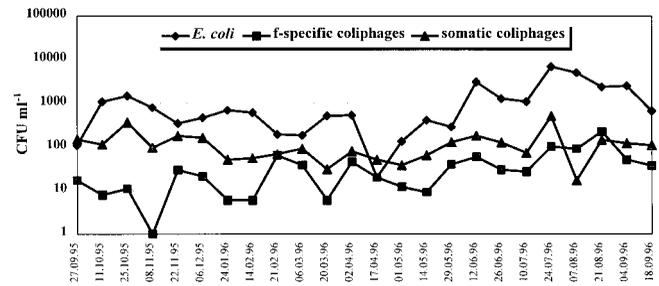
**Figure 8b** | Concentrations of *E. coli*, somatic and f-specific coliphages ( $\log cfu ml^{-1}$ ) in sewage effluent, results for the plant at HG.
