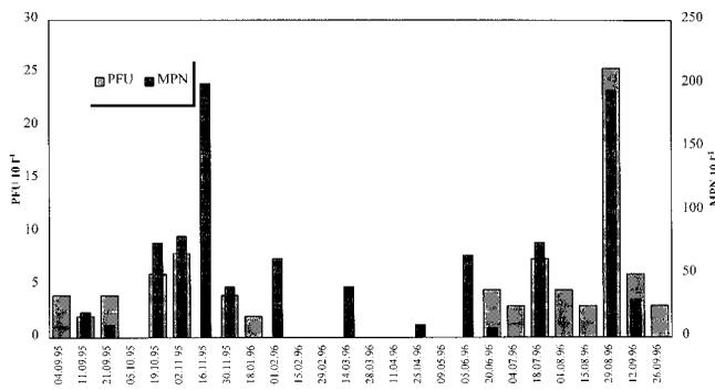
**Figure 3b** | Concentrations of viruses in sewage effluent ( $10 l^{-1}$ ), results for the plant at RT. The results given as PFU show concentrations of enteroviruses enumerated as plaque-forming-units, results given as MPN show concentrations of other enteric viruses enumerated as most probable number.
