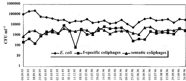
**Figure 4a** | Concentrations of *E. coli*, somatic and f-specific coliphages ( $\log cfu ml^{-1}$ ) in primary treated sewage, results for the plant at RT.
