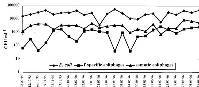
**Figure 6a** | Concentrations of *E. coli*, somatic and f-specific coliphages ( $\log cfu ml^{-1}$ ) in primary treated sewage, results for the plant at WE.
