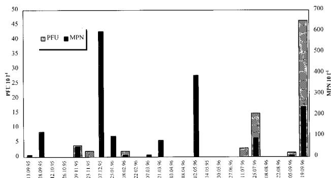
**Figure 5b** | Concentrations of viruses in sewage effluent ( $10 l^{-1}$ ), results for the plant at WE. The results given as PFU show concentrations of enteroviruses enumerated as plaque-forming-units, results given as MPN show concentrations of other enteric viruses enumerated as most probable number.
