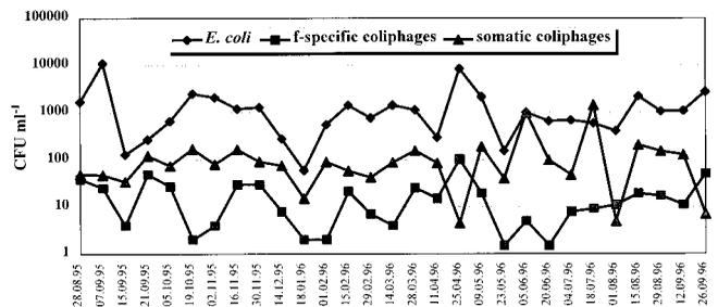
**Figure 2b** | Concentrations of *E. coli*, somatic and f-specific coliphages ( $\log cfu ml^{-1}$ ) in sewage effluent, results for the plant at Tü.
