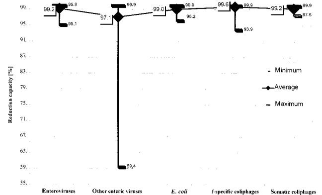
**Figure 9b** | Reduction capacities (%) for the different microorganisms at the RT plant with average, minimum and maximum reduction capacity.
