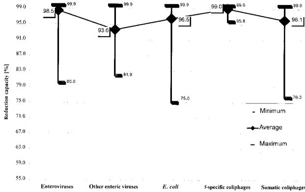
**Figure 9a** | Reduction capacities (%) for the different microorganisms at the TÜ plant with average, minimum and maximum reduction capacity.
