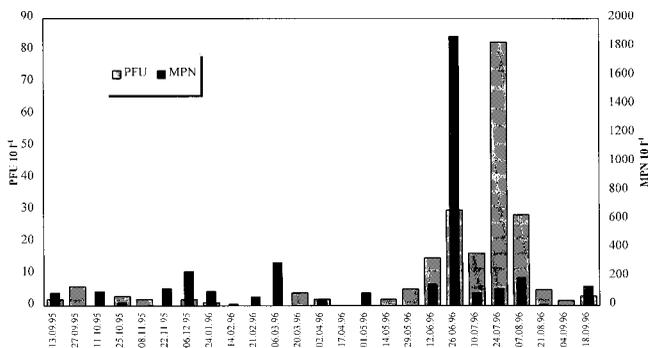
**Figure 7b** | Concentrations of viruses in sewage effluent ( $10 l^{-1}$ ), results for the plant at HG. The results given as PFU show concentrations of enteroviruses enumerated as plaque-forming-units, results given as MPN show concentrations of other enteric viruses enumerated as most probable number.
