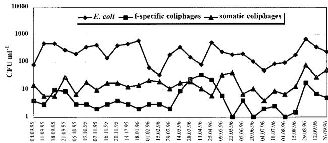
**Figure 4b** | Concentrations of *E. coli*, somatic and f-specific coliphages ( $cfu ml^{-1}$ ) in sewage effluent, results for the plant at RT.
