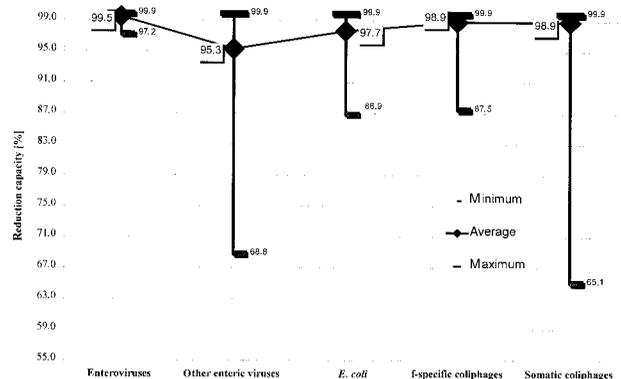
**Figure 9c** | Reduction capacities (%) for the different microorganisms at the WE plant with average, minimum and maximum reduction capacity.
