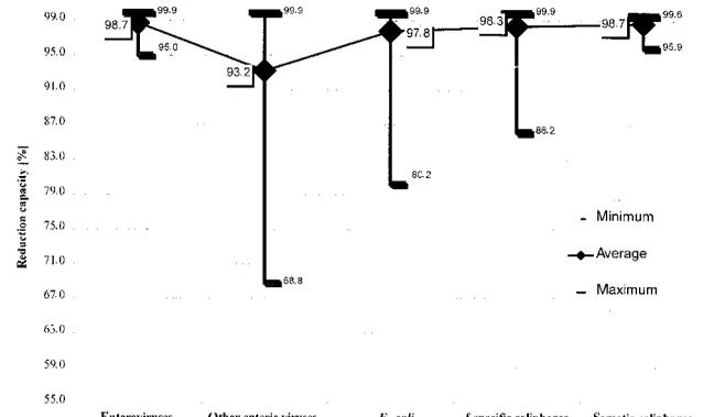
**Figure 9d** | Reduction capacities (%) for the different microorganisms at the HG plant with average, minimum and maximum reduction capacity.
