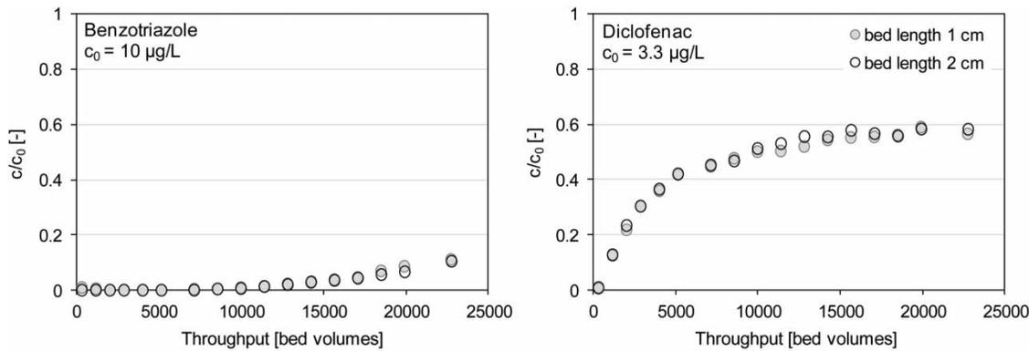
**Figure 2** | Benzotriazole and diclofenac concentrations, relative to the respective inlet WWTP effluent values, versus throughput of two RSSCTs with different bed length and different filter velocities ( $v_1 \sim 6$  m/h,  $v_2 \sim 12$  m/h) and same EBCT (6 s), GAC Norit 1240,  $d_p$ : 90–140  $\mu\text{m}$ .
