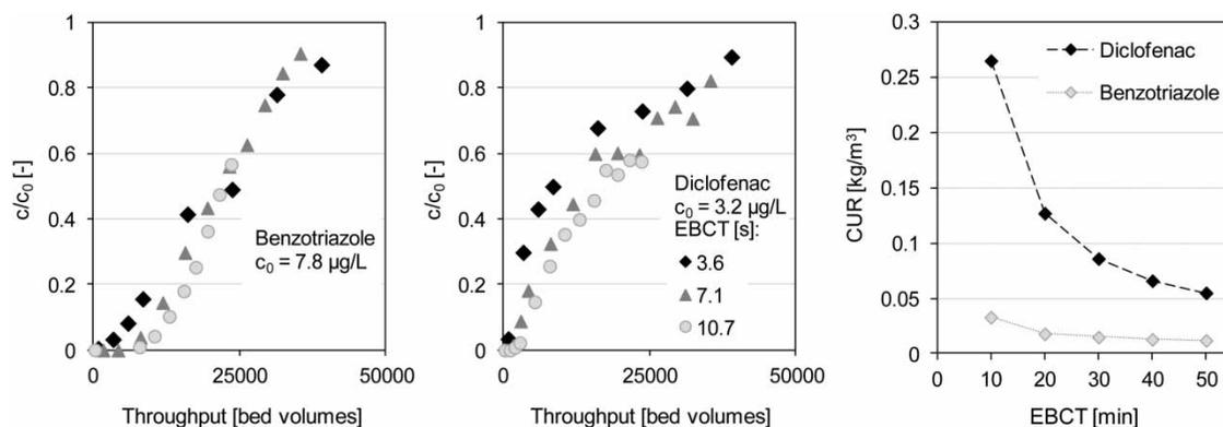
**Figure 4** | Left and middle: benzotriazole and diclofenac concentrations, relative to the inlet WWTP effluent values, versus throughput at varying EBCT,  $d_p$ : 90–140  $\mu\text{m}$ ; right: modeled CURs at 10% breakthrough for benzotriazole and diclofenac in relation to the EBCT.
