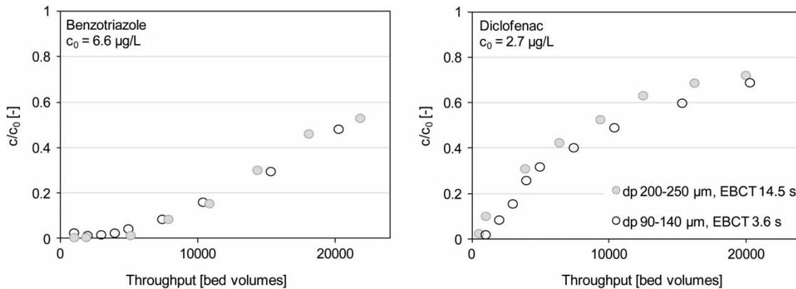
**Figure 3** | Benzotriazole and diclofenac concentrations, relative to the respective inlet WWTP effluent values, versus throughput in two equivalent RSSCTs with differently sized GAC and different EBCTs.
