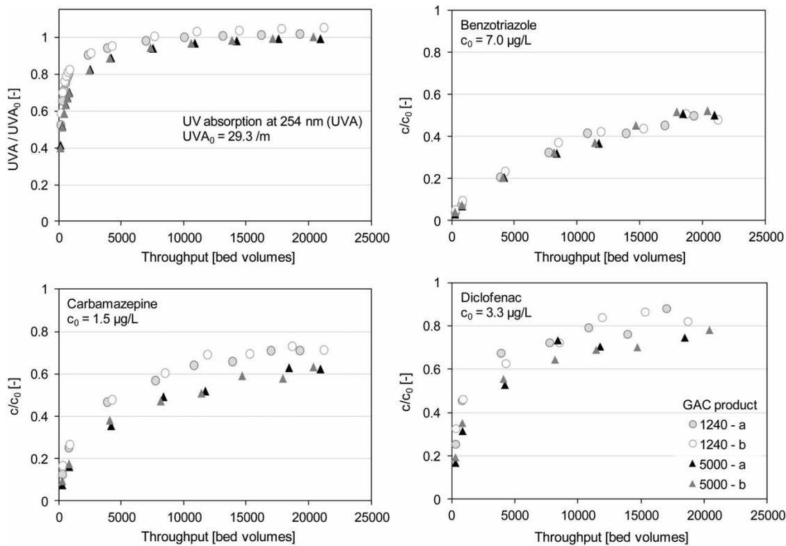
**Figure 1** | UV absorption and benzotriazole, carbamazepine, and diclofenac concentrations (relative to the respective inlet WWTP effluent values) versus throughput, with two different GAC products in duplicate (Norit 1240 and Aquasorb 5000), EBCT: 2.2 s,  $d_p$ : 125–200  $\mu\text{m}$ .
