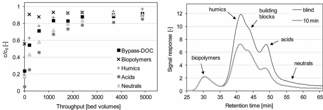
**Figure 5** | Left: DOC ('bypass-DOC') and DOC fraction concentrations, relative to the inlet WWTP effluent values, versus throughput; GAC AZ 1050,  $d_p$ : 125–200  $\mu\text{m}$ , EBCT (3 s); right: LC-OCD chromatograms of blind WWTP effluent sample and RSSCT outlet after 10 min, with fraction denominators (Huber et al. 2011).
