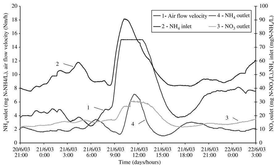
**Figure 5** FF/FB control at variable feed flow rate and constant recirculation ratio
