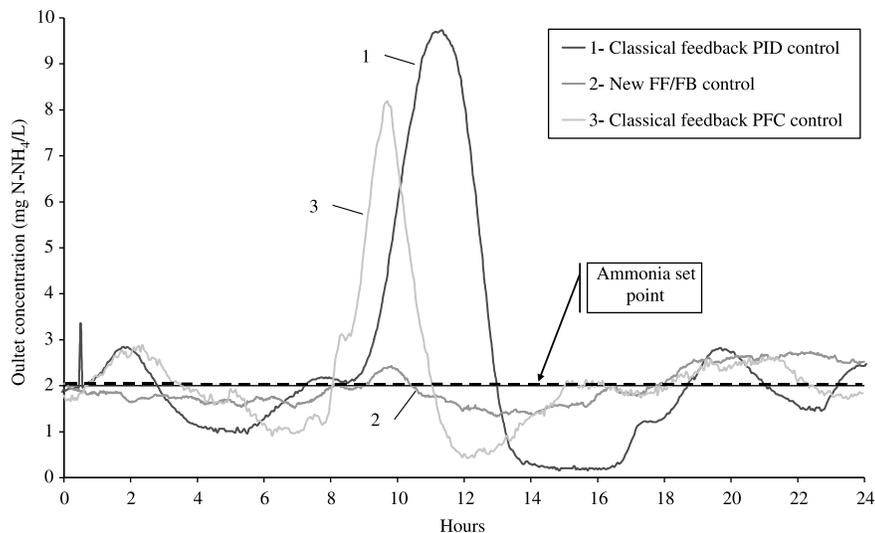
**Figure 4** Comparison of control concepts at constant flow rates,  $\text{NH}_4\text{-N}$  outlet
