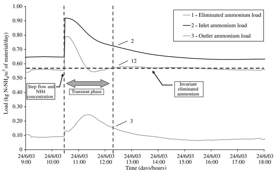
Figure 2 Results: Variation of  $\text{NH}_4\text{-N}$  conc. and feed flow rate at constant load
