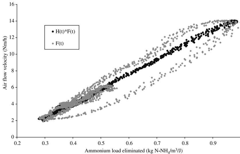
**Figure 3** Air flow velocity function of eliminated load value
