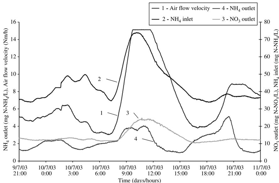
**Figure 6** FF/FB control at variable feed flow rate and variable recirculation ratio
