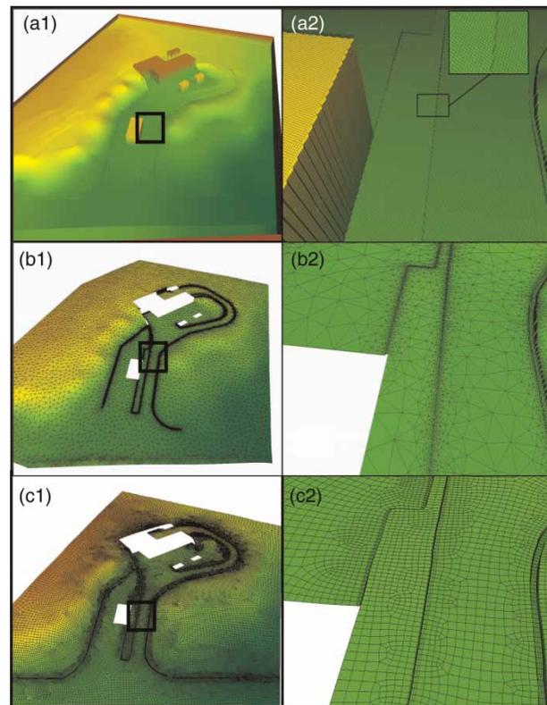
**Figure 3** | Mesh used in models (where: a1, a2 are Mike 21 grid views; b1, b2 are Mike 21 FM mesh views; c1, c2 are Néodyme 3D FVM mesh views).
