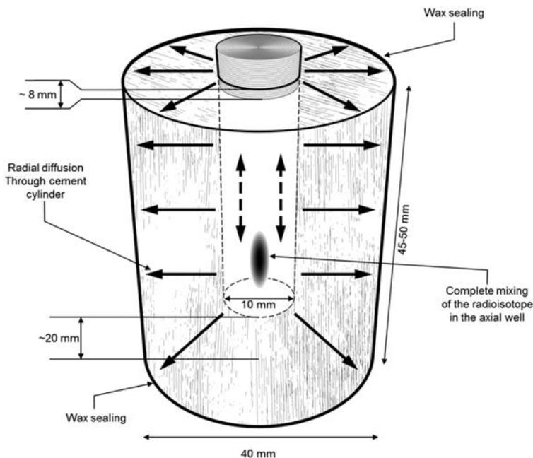
FIG. 1. Schematic of the radial diffusion experiments.
