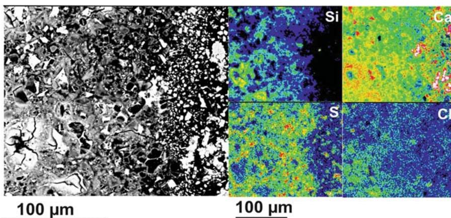
FIG. 7. Backscattered scanning electron microscope image of a partially hydrated calcium-silicate-sulfate cement clinker particle (left) with corresponding EDXA element distribution maps for Si, Ca, S and Cl. Higher concentrations of Cl are associated with the margins of this particle.
