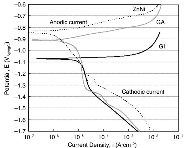
**FIGURE 10.** Polarization curves of coated steel sheets in 5 wt% NaCl solution under atmospheric conditions.
