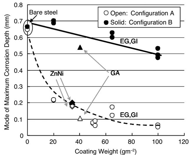
FIGURE 6. Effect of coating weight on corrosion depth on Configurations A and B at 60 cycles.
