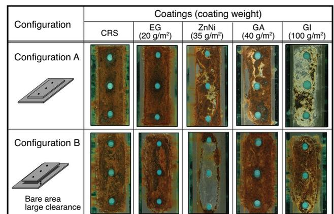
**FIGURE 5.** Appearance of disassembled specimens (large piece) of Configurations A and B at 60 cycles.
