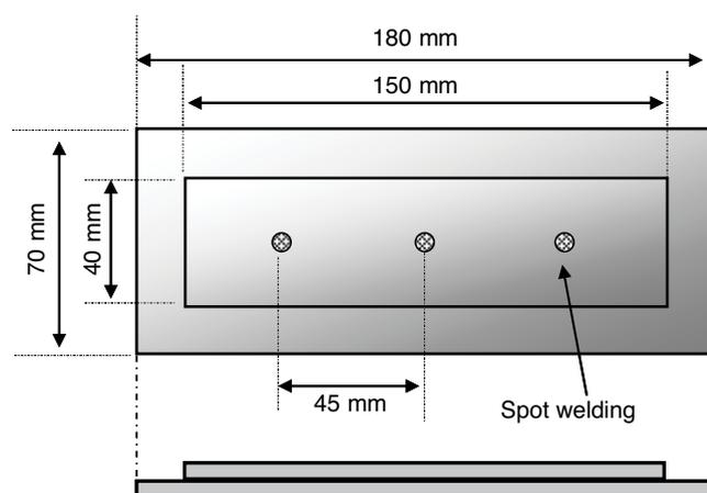
**FIGURE 1.** Configuration of lapped specimen for corrosion test.
