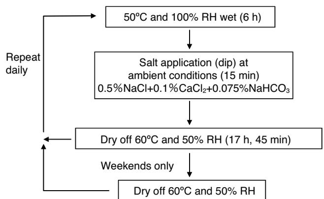
FIGURE 3. Test condition of SAE J2334—manual operation.
