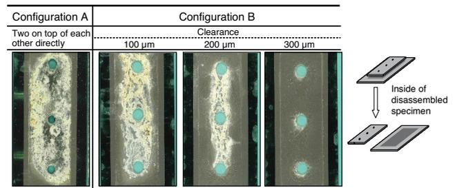
FIGURE 7. Appearance of disassembled GI 100 g/m<sup>2</sup> specimens (large piece) prepared without the spacers at 30 cycles.
