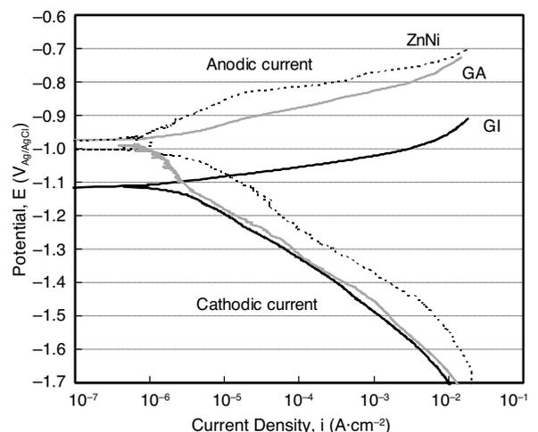
**FIGURE 11.** Polarization curves of coated steel sheets in deaerated 5 wt% NaCl solution.
