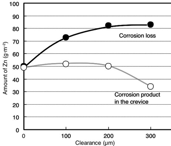
**FIGURE 8.** Corrosion loss and amount of corrosion product in the crevice as a function of clearance of lapped specimen at 60 cycles.
