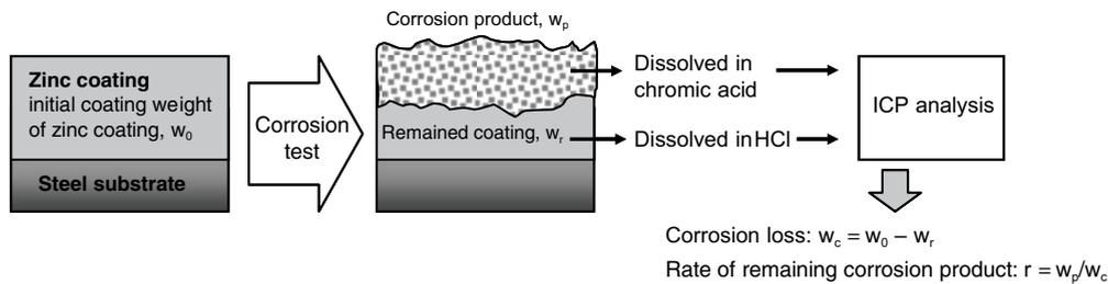
**FIGURE 4.** Determination of corrosion loss and the amount of remaining corrosion product by ICP analysis.
