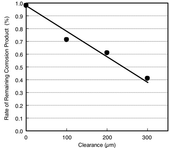
**FIGURE 9.** Rate of remaining corrosion product in the crevice as a function of clearance at 60 cycles.
