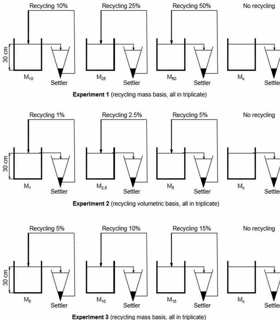
**Figure 1** | Schematic diagram for the operation of the HRAP mesocosms investigating the effect of different algal recycling rates on biomass productivity, settleability and *P. boryanum* dominance.
