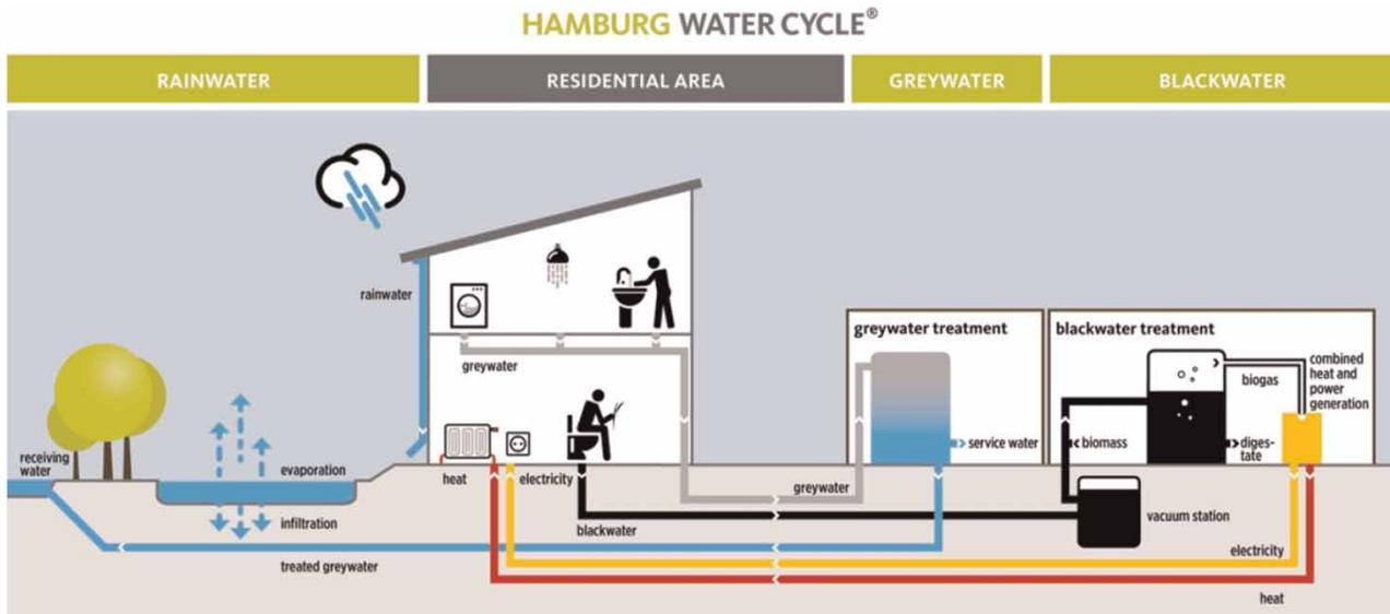
Figure 3 | HAMBURG WATER Cycle® – wastewater concept.
