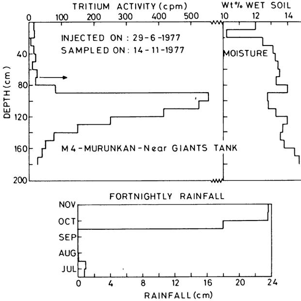
Fig. 10. Depth profiles of moisture contents and tritium activity from Murunkan, M4 (second phase). Fortnightly rainfall data for the intervening period are also given.
