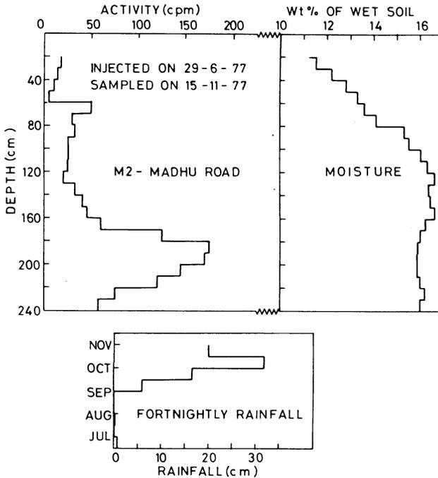
Fig. 9. Depth profiles of moisture contents and tritium activity from Madhu Road, M2 (second phase). Fortnightly rainfall data for the intervening period are also given.
