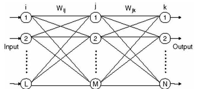
Figure 4 | A three layered feed-forward NN.
