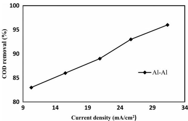
**Figure 4** | Effect of current density on COD removal efficiency.
