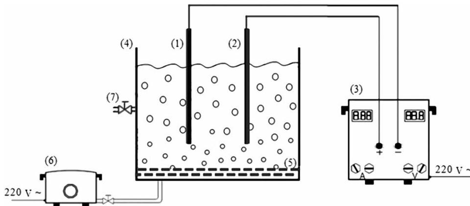
**Figure 1** | Schematic representation of the ECF set-up: (1) cathode, (2) anode, (3) DC power supply, (4) reactor, (5) perforated tube, (6) aeration pump and (7) sample port.
