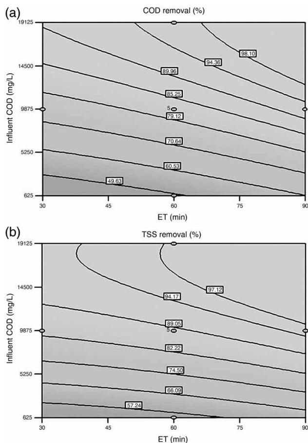
**Figure 6** | Effects of ET and influent COD on (a) COD and (b) TSS removal; voltage and ED are in the center of their domain (9,875 mg/L and 5 cm).
