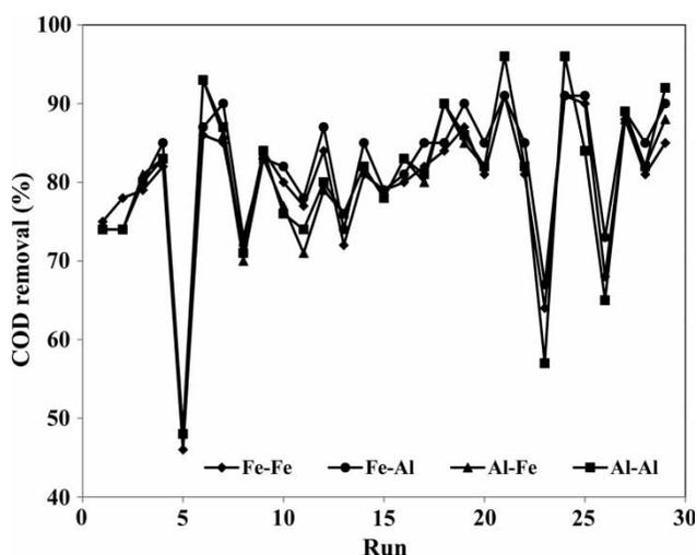
**Figure 2** | COD removal efficiency of different configurations (Al–Al, Al–Fe, Fe–Al, Fe–Fe) during all runs.
