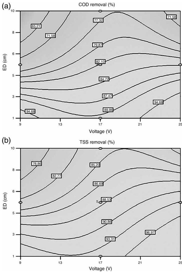
**Figure 3** | Effects of voltage and ED on (a) COD and (b) TSS removal; influent COD and ET are in the center of their domains (9,875 mg/L and 60 min).
