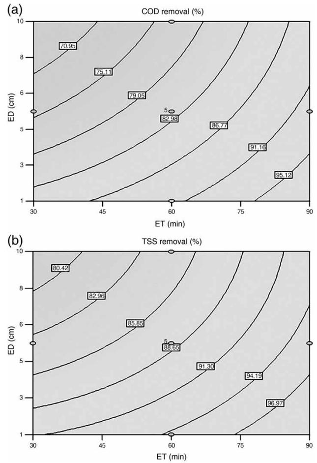
**Figure 5** | Effects of ED and ET on (a) COD and (b) TSS removal; influent COD and voltage are in the center of their domain (9,875 mg/L and 17 V).
