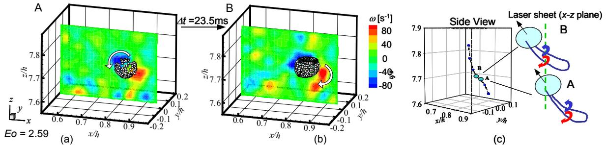
**FIG.2 THREE DIMANSIONAL BUBBLE SHAPE AND CORRESPONDING FLOW STRUCTURE, (a) Instantaneous Bubble Shape and Vorticity Contour at Position A, (b) Instantaneous Bubble Shape and Vorticity Contour at Position B, (c) Three Dimensional Bubble Trajectory (Side View).**
