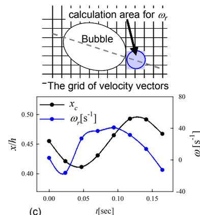
**FIG.3 THE RELATION BETWEEN BUBBLE DEFORMATION AND WAKE STRUCTURE, (a) Definition of Asymmetric Property Parameter  $R_l$  and Relation between Aspect Ratio  $As$  and  $R_l$ , (b) Schematic of Deformed Bubble Motion, (c) Relation between  $x_c/h$  and  $\omega_r$ .**
