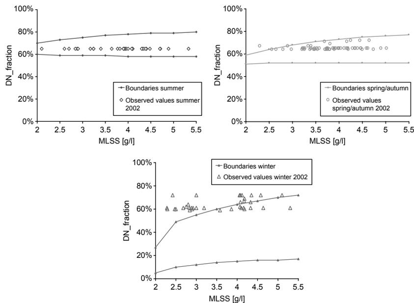
**Figure 2** Operability space of the nitrification/denitrification process: boundary conditions for MLSS and the DN fraction and values observed in 2002 at WWTP Ertvelde
