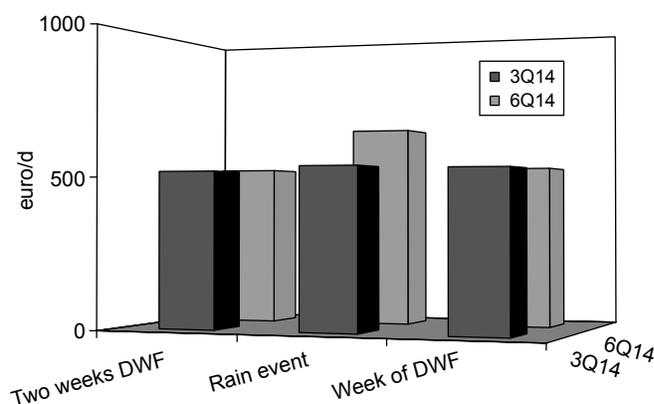
Figure 6 Comparison of the total costs for  $3Q_{14}$  and  $6Q_{14}$  operational strategies WWTP Boom
