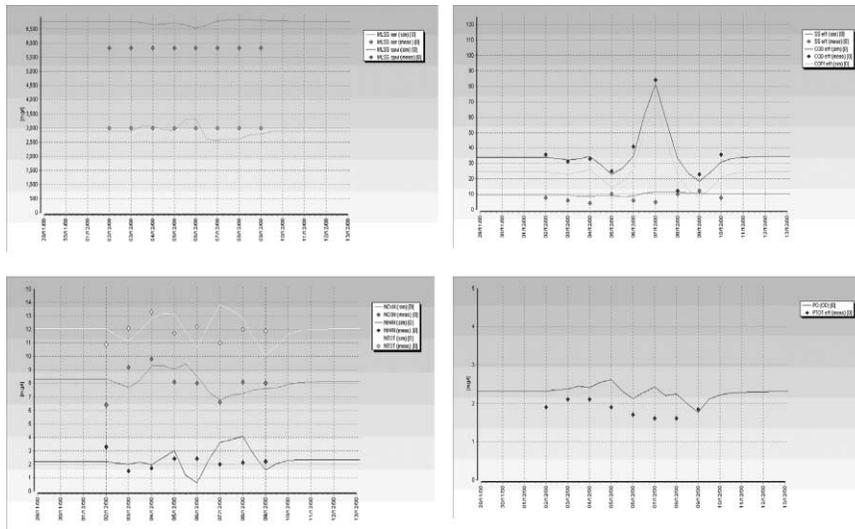
**Figure 1** Results of validation for WWTP Eksel: (a) MLSS concentration in the aeration and in the return, (b) COD, COD filtered and suspended solids in the WWTP effluent, (c)  $\text{NH}_4\text{-N}$ ,  $\text{NO}_3\text{-N}$  and total nitrogen in the WWTP effluent, (d) total phosphorus in the WWTP effluent (lines: simulations; points: observations)
