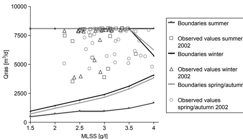
**Figure 3** Operability space of the sedimentation process: boundary conditions for MLSS and Qras and values observed in 2002 at WWTP Achel
