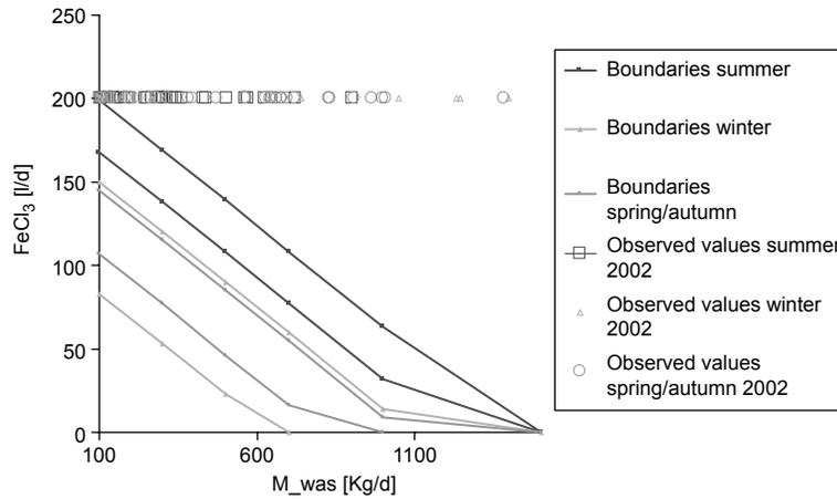
**Figure 4** Operability space of chemical phosphorus precipitation: boundary conditions for the sludge production ( $M_{\text{was}}$ ) and the dosing rate of  $\text{Fe}^{3+}$  products and values observed in 2002 at WWTP Heist op den Berg
