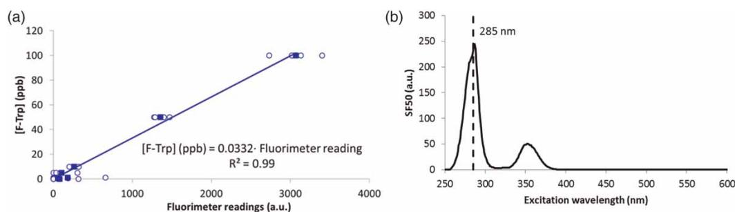
**Figure 1** | (a) Calibration curve for tryptophan on the SMF4. Closed symbols = mean of four readings (open symbols) for each concentration;  $R^2$  = coefficient of determination for the linear correlation based on the mean values; (b) SF50 spectrum of a solution of tryptophan in ultra-pure water. The band at  $\lambda_{exc} \approx 350$  nm is due to water.
