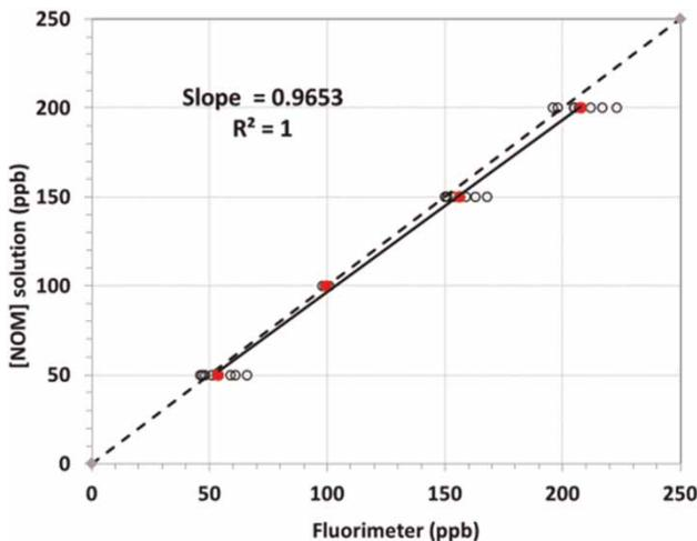
**Figure 2** | Calibration of the 10AU against quinine sulfate, surrogate substance for NOM. Closed symbols = average of eight readings (open symbols) for each concentration;  $R^2$  = coefficient of determination for the linear correlation based on the mean values.
