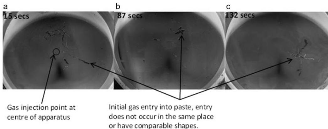
FIG. 2. First image showing gas entering the clay paste and time since initiation of injection (note varying times and textures in each test showing inconsistency of gas entry). (a) Test FVR\_K01; ring highlights gas point of injection from beneath, (b) Test FVR\_K02, (c) Test FVR\_K03.
