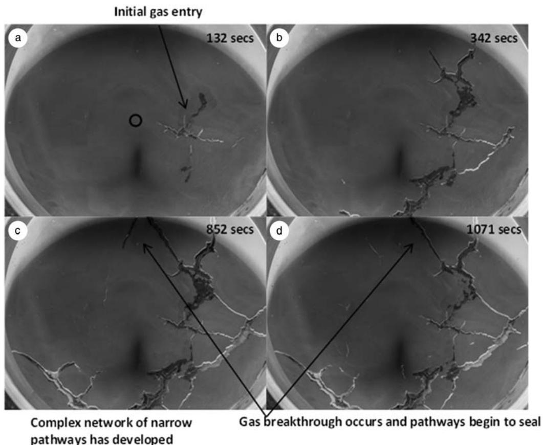
FIG. 5. Images showing evolution of Test FVR\_K03 with respect to time. (a) Initial gas entry in isolated position, gas injection point shown by ring; (b) development of dilatant pathways away from point of entry; (c) large pathway to bottom left of image reaches edge of apparatus, resulting in gas breakthrough and decrease of gas pressure in pathways; and (d) once gas breakthrough occurs, pathways away from point of breakthrough begin to close, as shown by label.
