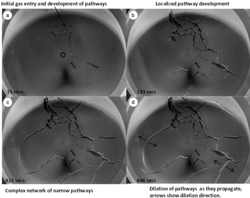
FIG. 3. Evolution of Test FVR\_K01 over time. (a) Initial gas entry, ring shows gas injection point, (b) Localized pathways begin to develop, (c) Development of network of pathways gives dendritic texture, (d) Larger pathways can be seen to dilate as gas pressure increases, shown by arrows on image.
