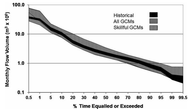
**Figure 9** | Flow duration curve envelopes (the upper and lower bounds of 90% of the simulation ensembles) for the near future for all GCMs and the three most skilful, as well as the simulations using historical data.
