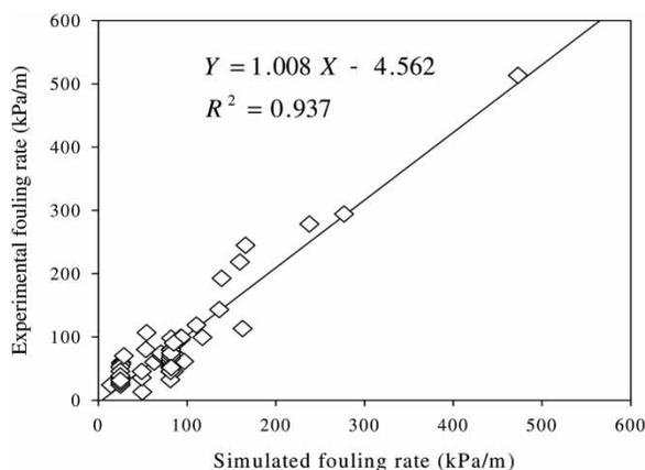
**Figure 4** | Simulated membrane fouling rate vs. experimental measurement.
