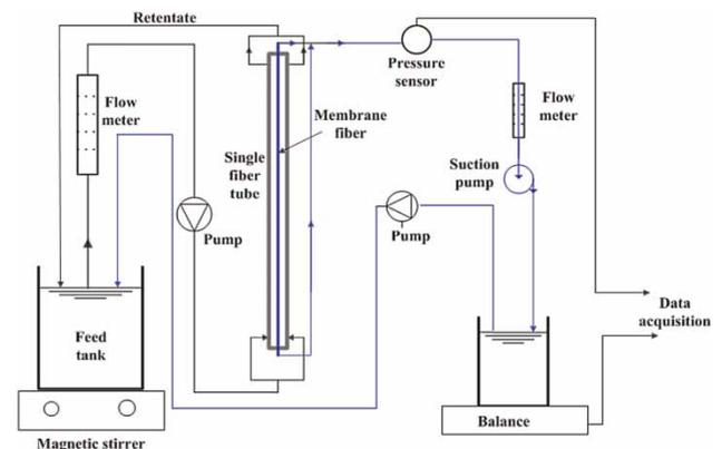
Figure 1 | Schematic of the single-fibre MF testing system.
