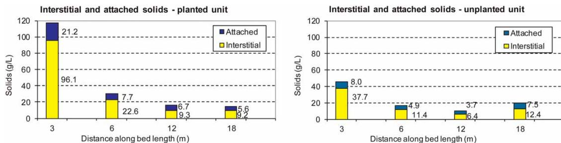
Figure 4 | Proportion of interstitial and attached solids along the bed in the planted and unplanted units.
