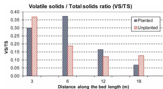
**Figure 3** | Ratio of volatile and total solids along the planted and unplanted units.
