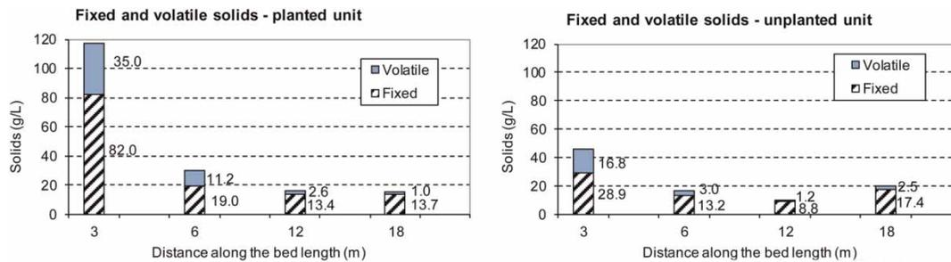
**Figure 2** | Distribution of fixed and volatile solids along the bed length of the planted and unplanted units.
