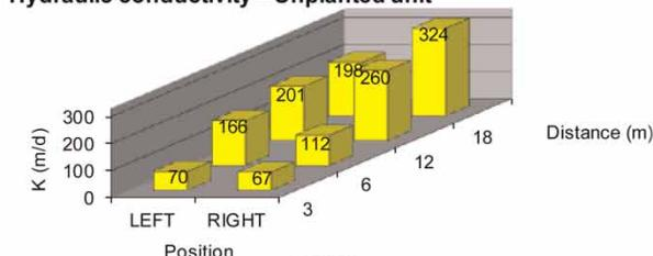
Figure 6 | Distribution of hydraulic conductivity in the filter medium along the planted wetland PW (left chart) and unplanted UPW (right chart).
