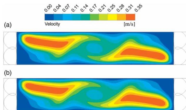
Figure 4 | Comparison of velocity color contour diagrams comparing the periodic and non-periodic solutions.
