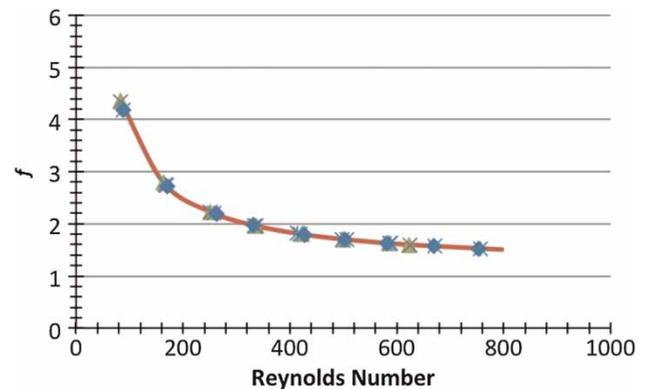
**Figure 7** | Comparison of the numerical predictions, based on the measured dimensions of the flow passage, with the experimental data. The predictions are represented by the continuous curve and the experiments by the discrete points.
