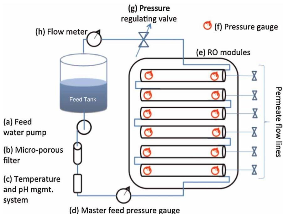
Figure 1 | Schematic diagram of the experimental facility.
