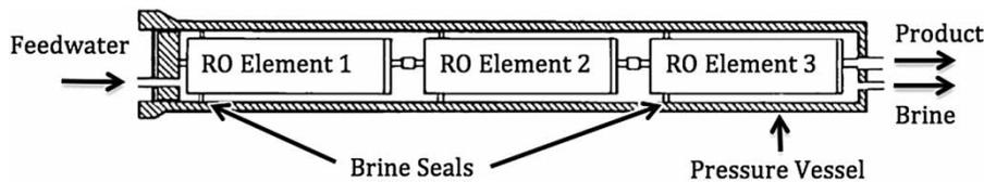
Figure 2 | Schematic diagram of an RO pressure vessel.
