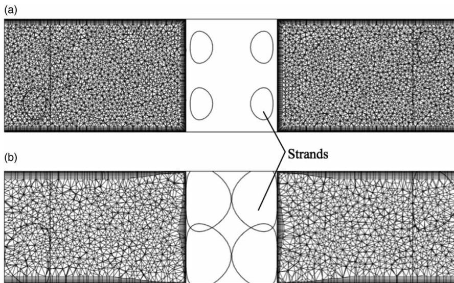
**Figure 6** | Meshes for the geometries based on (a) manufacturer's specifications and (b) actual intruded geometry.
