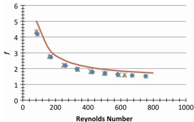
Figure 5 | Comparison of the numerical predictions, based on the manufacturer-indicated dimensions of the flow passage, with the experimental data. The predictions are represented by the continuous curve and the experiments by the discrete points.
