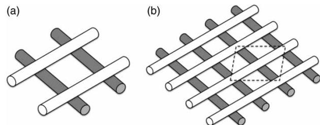
Figure 3 | Illustrations of non-woven feed spacers. (a) A single pair of spacers and (b) an array of spacers (the box shows the 'repeating unit' used for CFD simulation).
