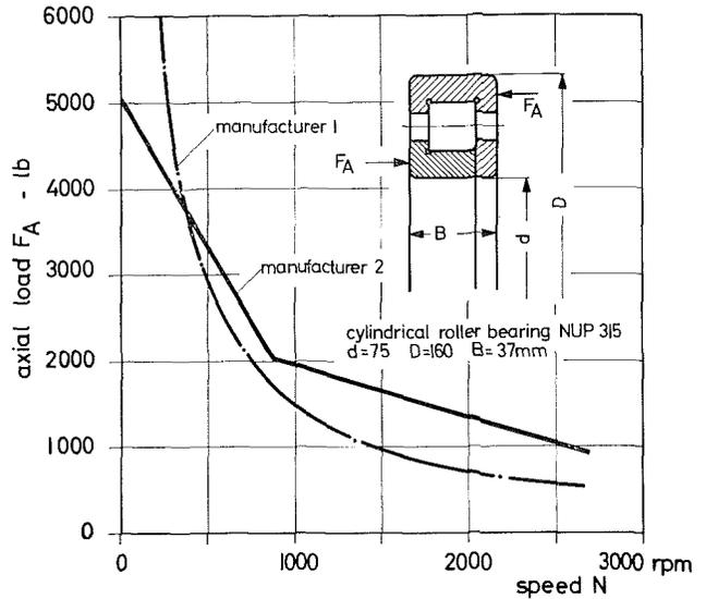
Fig. 13 Safe thrust load by conventional calculation
