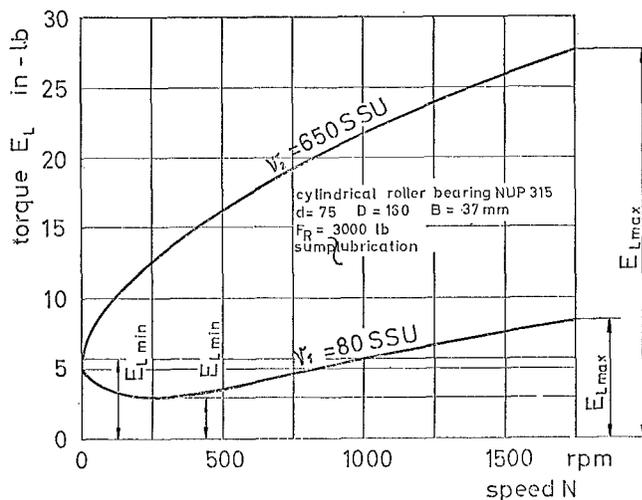
Fig. 20 Bearing friction of different viscosities and speeds
