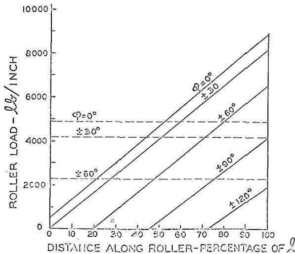
Fig. 18 Roller loading versus axial and circumferential location
