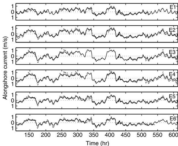
**Figure 5** | Measured (symbols) and modelled (lines,  $\beta = 0.055$ ,  $k_a = 0.026$  m and  $\nu = 1.30$  m<sup>2</sup> s<sup>-1</sup>)  $\bar{v}$  from offshore (E1) to onshore (E6) versus time at Egmond.
