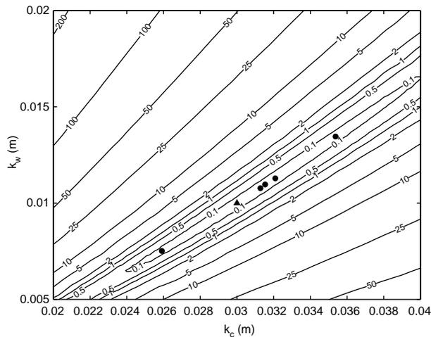
**Figure 9** | Contour plot of the objective function  $F$  for the synthetic bathymetric data as a function of the current-related roughness  $k_c$  and the wave-related roughness  $k_w$  ( $\tan \phi = 0.2$ ). The triangle is located at the known optimum,  $k_c = 0.03$  m and  $k_w = 0.01$  m. The circles are the solutions of the GA-SX algorithm.
