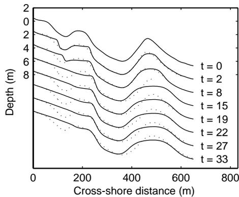
**Figure 11** | Measured (dotted lines) and modelled (solid lines,  $k_c = 0.03$  m,  $k_w = 0.011$  m and  $\tan \phi = 0.25$ ) bed evolution data set. The time stamp refers to the number of days after the initial depth profile. Each consecutive profile is offset by an additional 2 m.
