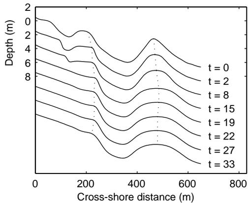
**Figure 7** | Synthetic bed evolution data set. The time stamp refers to the number of days after the initial depth profile. Each consecutive profile is offset by an additional 2 m. The dotted lines connect the inner and outer bar crest positions, respectively.
