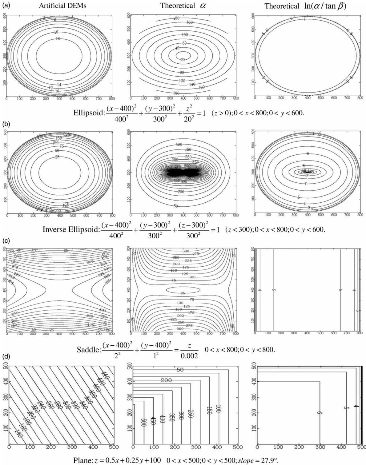
**Figure 6** | Contour maps. Left column: artificial DEM surfaces; middle column: the theoretical  $\alpha$  distributions; and right column: the theoretical  $\ln(\alpha/\tan \beta)$  distributions of four typical mathematical surfaces: (a) ellipsoid; (b) inverse ellipsoid; (c) saddle; and (d) plane. These plots provide the standard ‘true’ values of  $\alpha$  and  $\ln(\alpha/\tan \beta)$ , which are taken as the evaluating benchmarks for calculating the MFD and NMFD algorithm errors.
