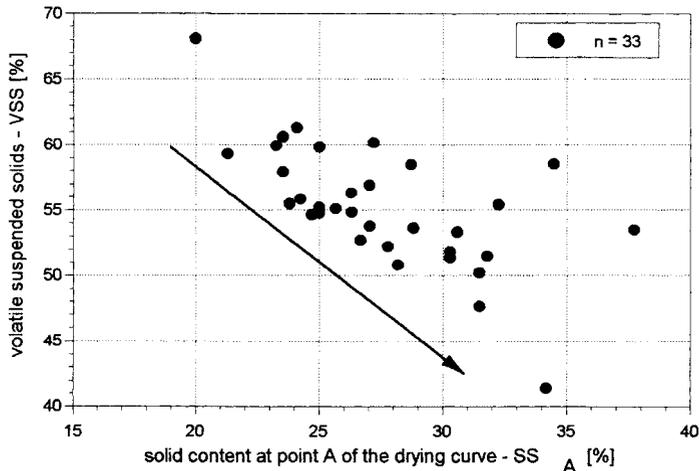
**Figure 8** Dependency of the achievable dewatering results  $SS_A$  on the volatile suspended solids
