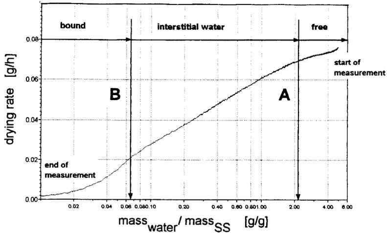
**Figure 2** Drying curve of a digested sewage sludge for a logarithmic abscissa
