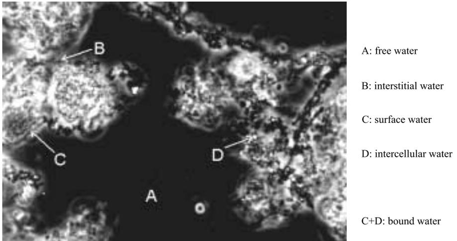
**Figure 1** Water distribution in a sewage sludge floc
