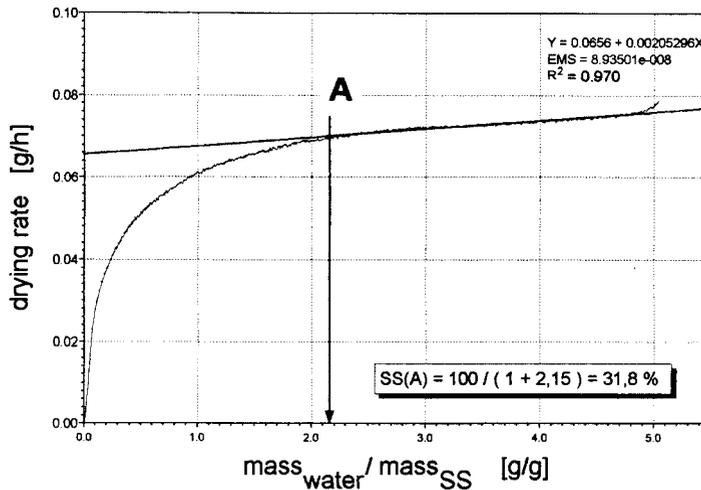
**Figure 3** Drying curve of a digested sewage sludge for an arithmetic abscissa
