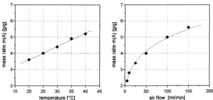
Figure 4 Dependence of the drying curve on laboratory conditions
