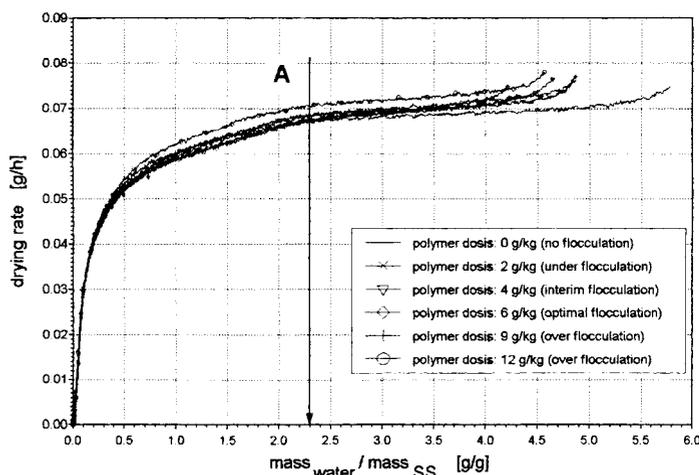
**Figure 7** Influence of polymer conditioning on the drying curve
