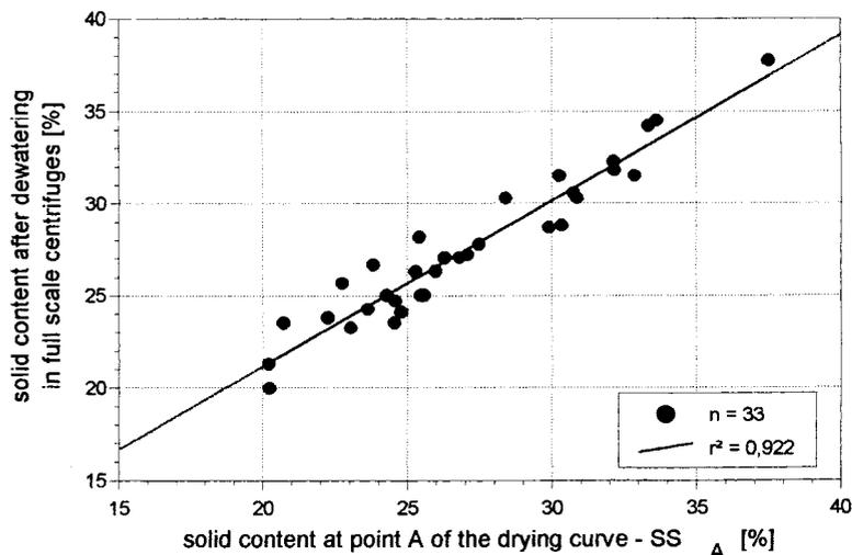
**Figure 6** Correlation between  $SS_A$  solid content at point A of the drying curve in dependence of the solid contents after dewatering in full scale centrifuges
