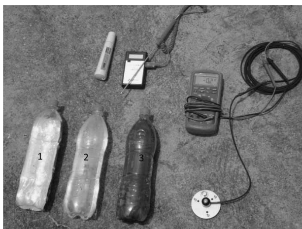
Figure 1 | Polyethylene terephthalate (PET) bottles with (1) reflective, (2) transmissive and (3) absorptive backing surfaces.
