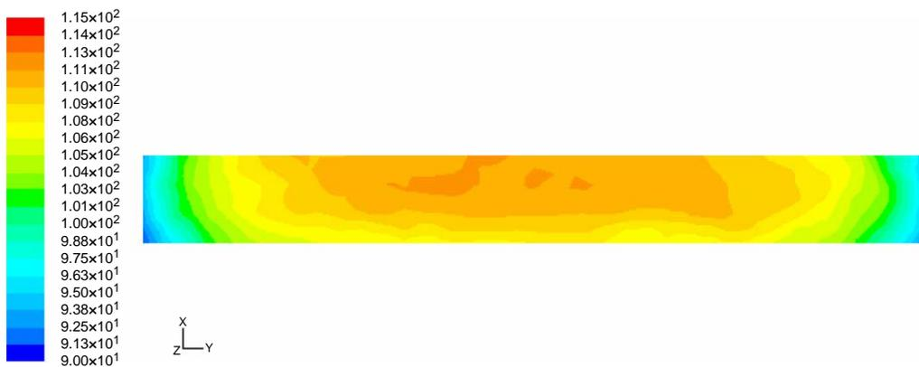
**Figure 7** | UV irradiance ( $\text{W/m}^2$ ) computed by the CFD simulation on the quartz plate above the catalyst-coated slides.
