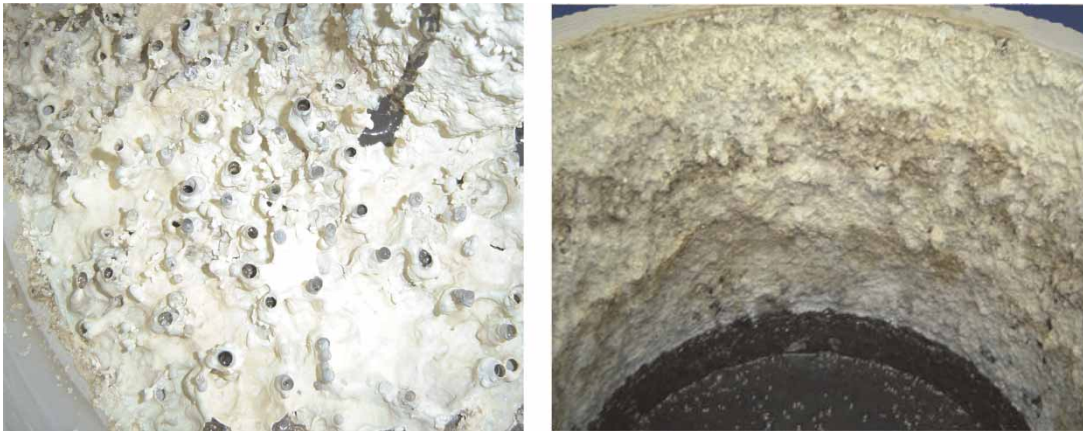
Figure 4 | Sulfur deposition in the headspace. Left: top of the reactor. Right: walls above the liquid surface.
