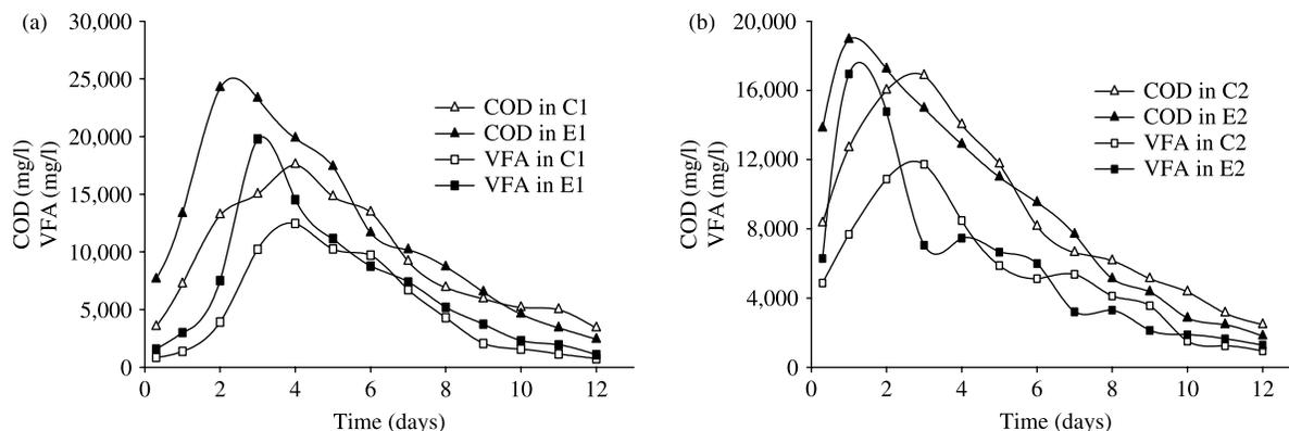
**Figure 3** | Changes in concentration of COD and VFA in control (C) and experiments (E) for thermally treated waste (a) and frozen/thawed waste (b).
