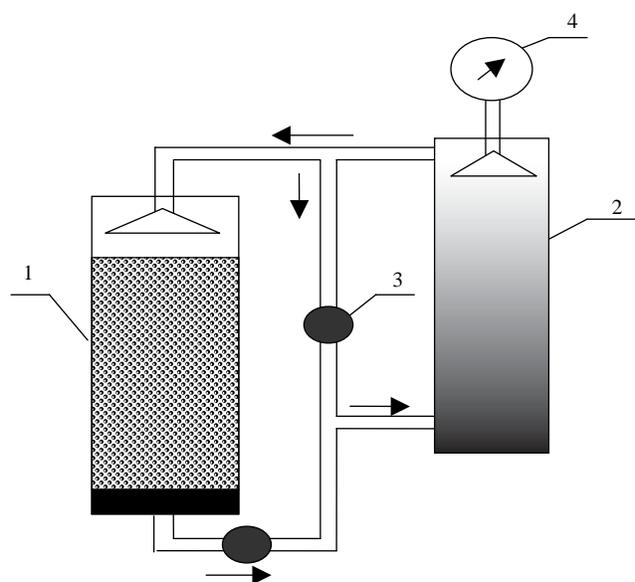
**Figure 1** | Schematic diagram of the HASL system: 1, acidogenic reactor, Ra; 2, methanogenic reactor, Rm; 3, peristaltic pump; 4, wet gas meter.
