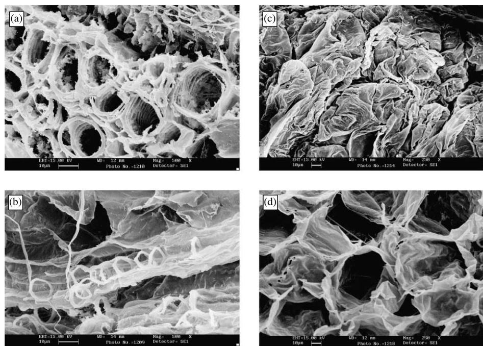
**Figure 2** | SEM images of fresh (a) and thermally pre-treated (b) vegetable waste; of fresh (c) and frozen/thawed (d) vegetable waste.
