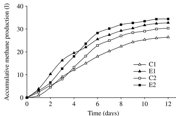
**Figure 4** | Accumulative methane productions in control (C) and experiments (E) for thermally treated waste (1) and frozen/thawed waste (2).
