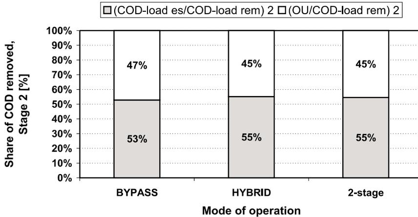
**Figure 7** Pathways of COD-removal of the second stage. Shares of COD-load removed by means of excess sludge withdrawal from the second stage (COD-load es, pumped into the first stage) and respiration (OU) respective to the total removed COD-load (COD-load rem) of the second stage
