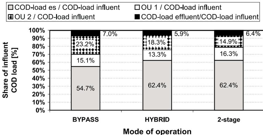
**Figure 6** Pathways of COD-removal of the entire plant. Shares of COD-load removed by means of excess sludge withdrawal from the first stage (COD-load es), respiration in both stages (OU I, OU II) and COD effluent load (COD-load effluent) respective to the COD influent load (COD-load influent) to the plant
