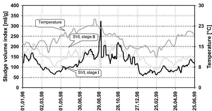
**Figure 9** Sludge volume index and temperature during the course of operation of the pilot plant
