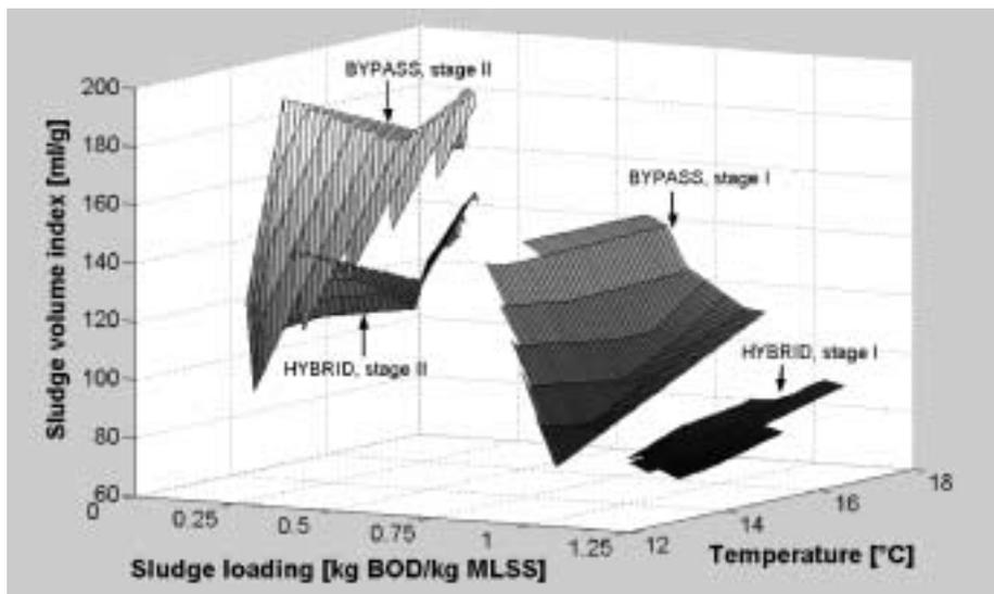
**Figure 8** Sludge volume index of the two stages of the pilot plant at main Vienna STP during different operational modes
