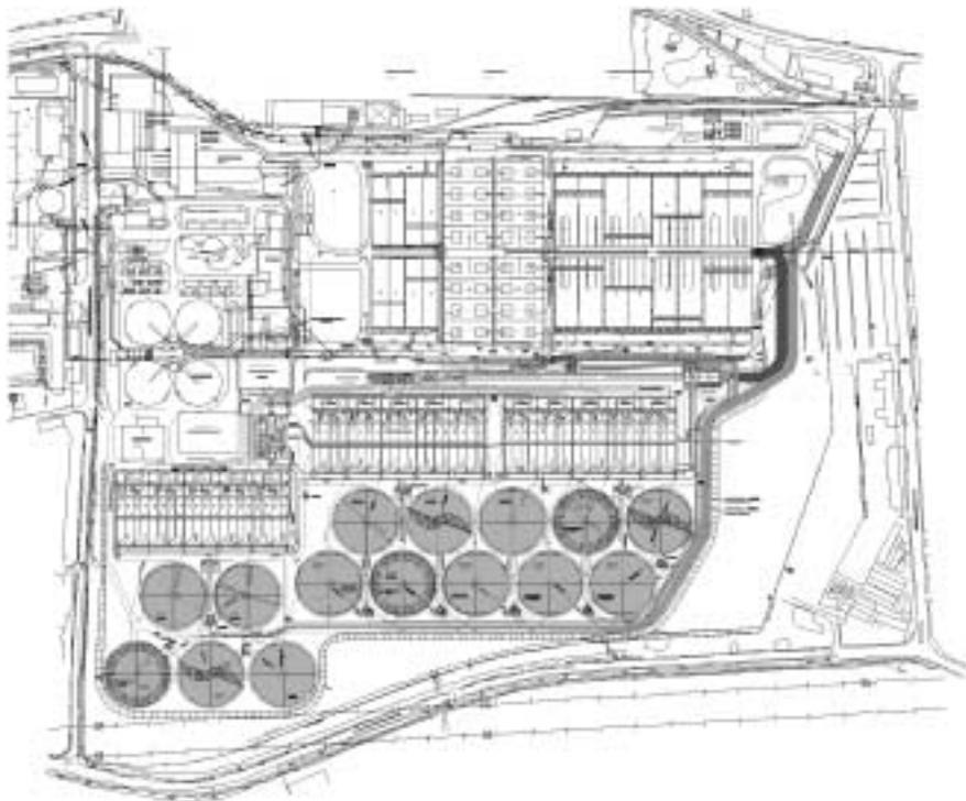
**Figure 1** Vienna STP existing plant (upper part) and plant extension (lower part, under construction)
