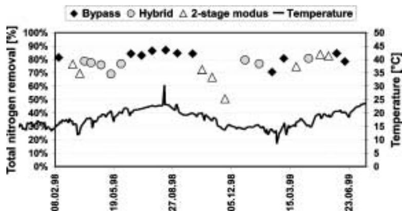
**Figure 3** Nitrogen removal performance of the pilot plant during different operational periods
