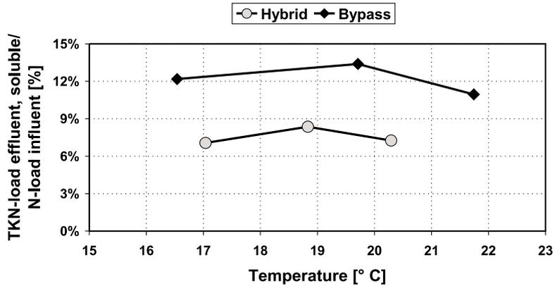
**Figure 5** Percentage of soluble TKN in the effluent relative to the total nitrogen influent load during Bypass- and Hybrid®-operation
