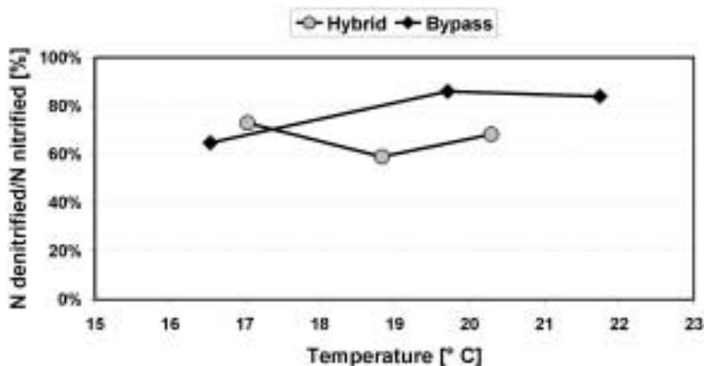
**Figure 4** Percentage of denitrified nitrogen load relative to the nitrified nitrogen load during Bypass- and Hybrid<sup>®</sup>-operation
