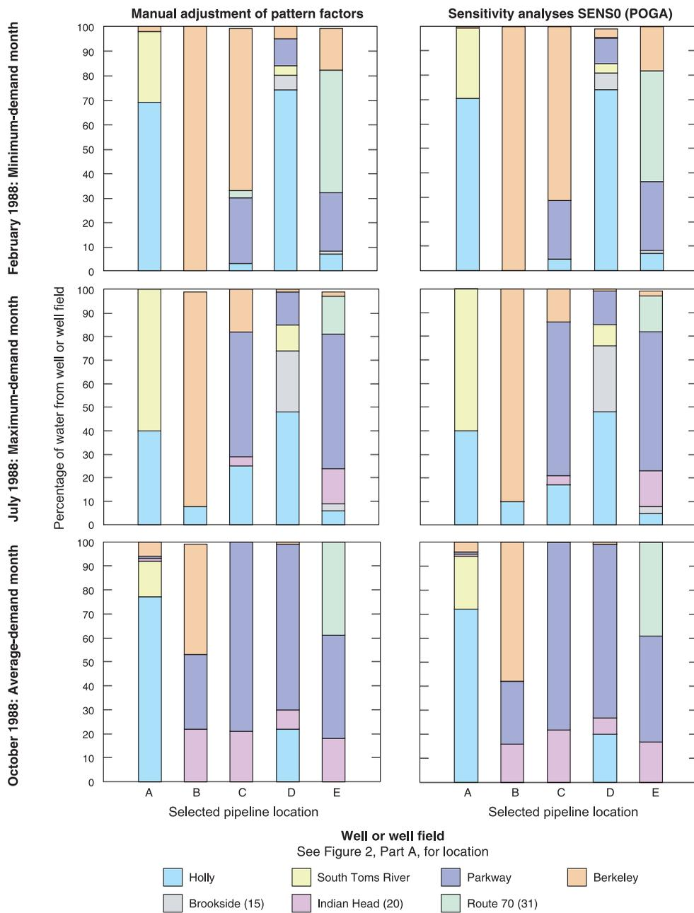
**Figure 16** | Simulated proportionate contribution of water derived from the manual adjustment of pattern factors and sensitivity analyses SENS0 for selected pipeline locations, Dover Township area, New Jersey, February, July and October 1988 (number in parenthesis is individual well number) (from Maslia *et al.* 2001).
