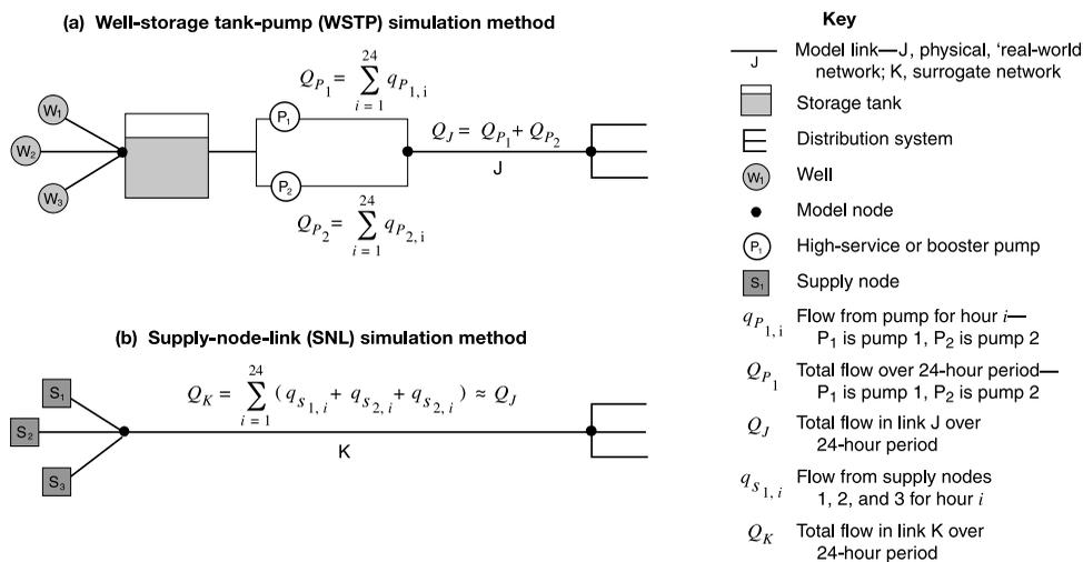
**Figure 1** | Distribution system representation of supply well, storage tank and pump combination for (a) physical 'real-world' network and (b) model network used for historical reconstruction analysis (from Maslia *et al.* 2001).
