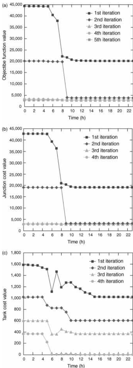
**Figure 10** | Convergence of (a) objective function as a function of iteration number and time step, (b) junction cost as a function of iteration number and time step, (c) tank cost as function of iteration number and time step, October 1996 (from Maslia et al. 2001).
