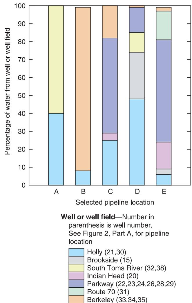
**Figure 3** | Simulated proportionate contribution of water from wells and well fields to selected locations using the manually adjusted supply-well and supply-node pattern factors, Dover Township area, New Jersey, July 1988 (from Maslia *et al.* 2001).
