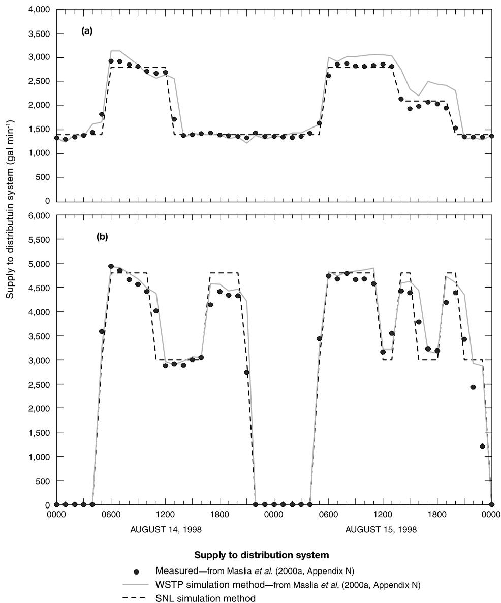
**Figure 2** | Measured and simulated flows using the well-storage tank-pump (WSTP) and supply-node-link (SNL) simulation methods, Dover Township area, New Jersey, August 1998 at (a) Holly Plant facility and (b) Parkway facility (from Maslia *et al.* 2001).
