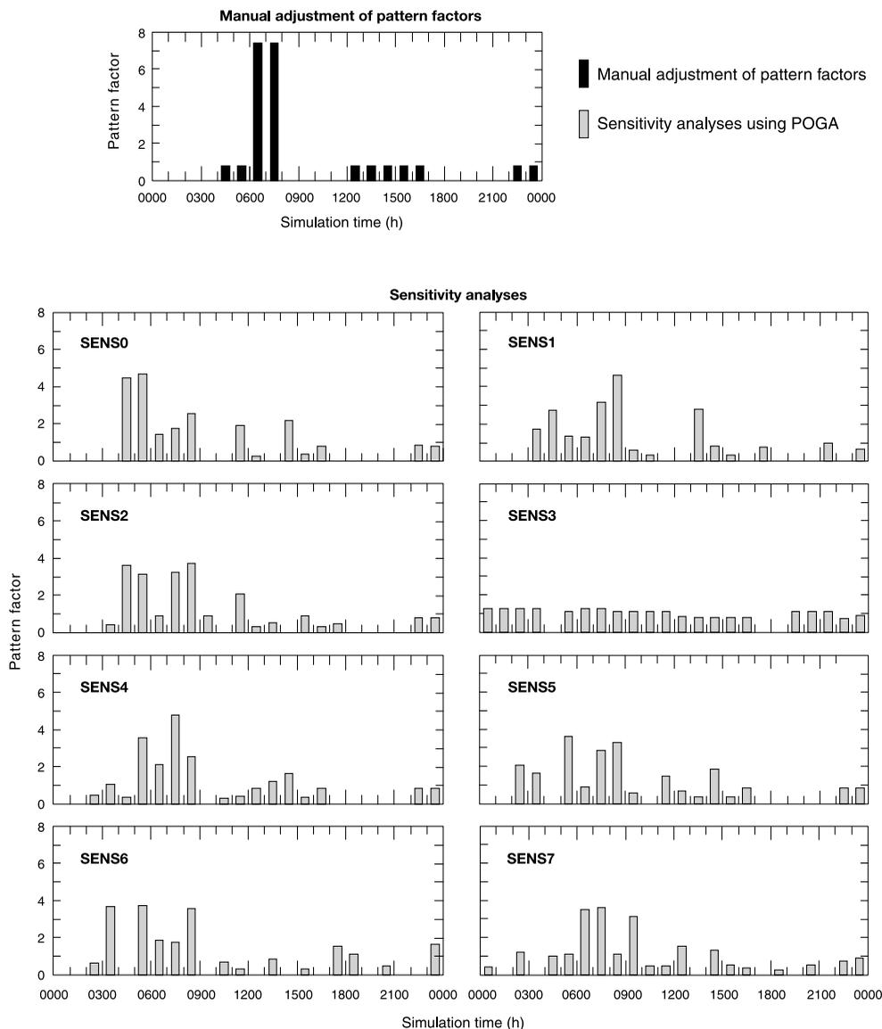
**Figure 17** | Pattern factors derived using manual adjustment and sensitivity analyses (POGA), supply node represents Parkway well 22, October 1996 conditions (see Figure 2, Part A for well location) (from Maslia *et al.* 2001).
