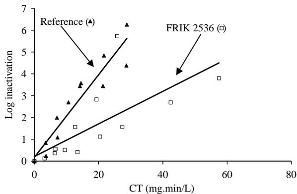
**Figure 8** | Inactivation by monochloramine (pH 8.0, 21°C) of *E. coli* O157:H7 ATCC 35150 (▲) and *E. coli* O157:H7 FRIK 2536 (□) strains.
