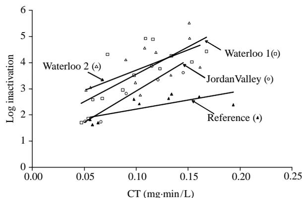
Figure 1 | Chlorine inactivation (pH 7.0, 25°C) of *B. vesicularis*.
