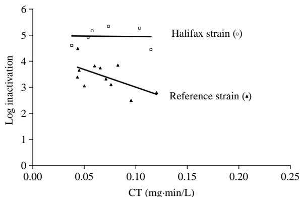
Figure 2 | Chlorine inactivation (pH 7.0, 25°C) of *P. fluorescens*.
