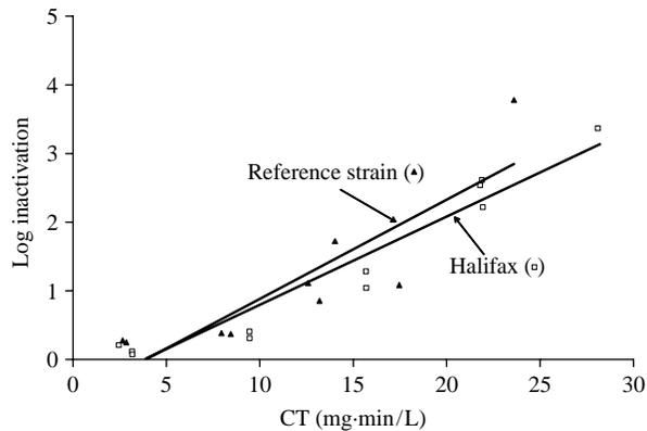
Figure 5 | Monochloramine inactivation (pH 8.0, 25°C) of *P. fluorescens*.
