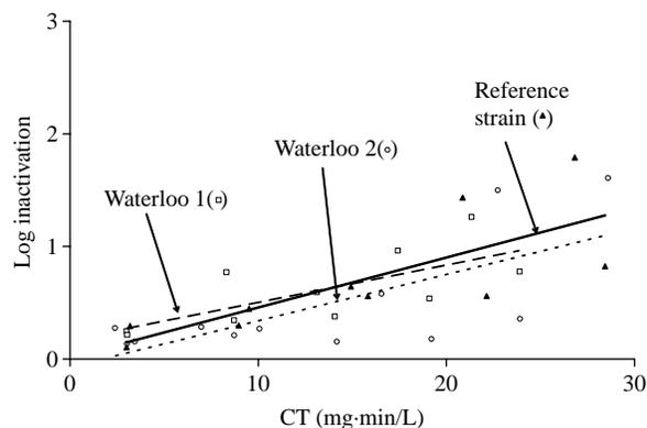
**Figure 4** | Monochloramine inactivation (pH 8.0, 25°C) of *B. vesicularis*.
