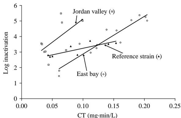
**Figure 3** | Chlorine inactivation (pH 7.0, 25°C) of *S. paucimobilis*.
