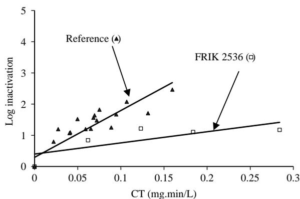
**Figure 7** | Inactivation by free chlorine (pH 7.0, 21°C) of *E. coli* O157:H7 ATCC 35150 (▲) and *E. coli* O157:H7 FRIK 2536 (□) strains.
