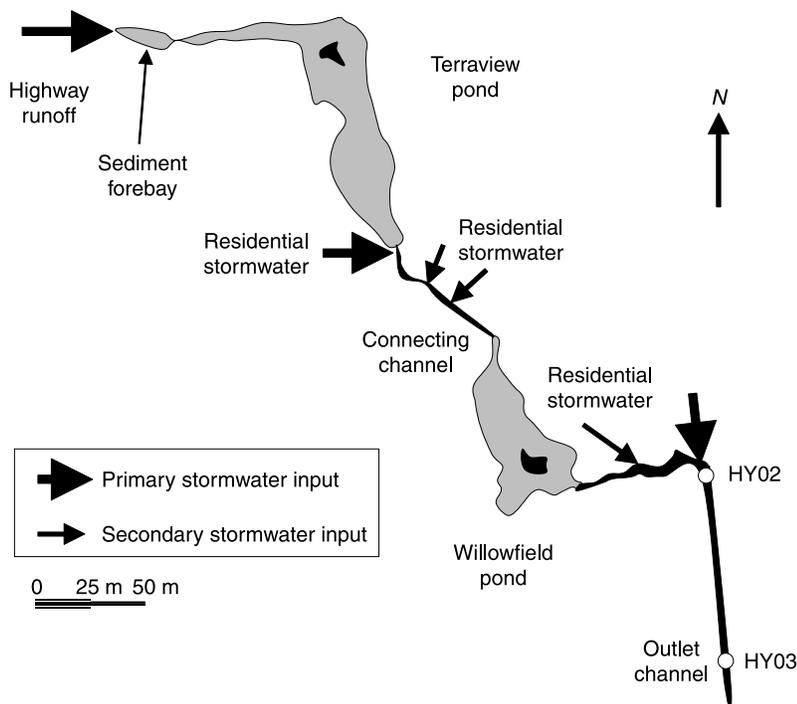
**Figure 1** | Layout of the Terraview-Willowfield Stormwater Management Park (TWSMP) in Toronto, Canada.
