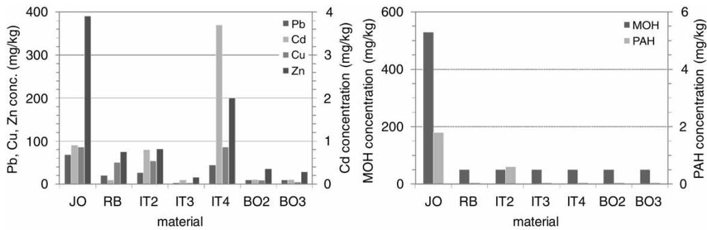
Figure 5 | Particle concentrations with regard to heavy metals (left side) and hydrocarbons (right side).
