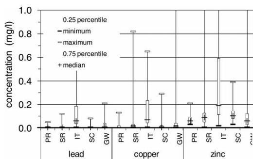
**Figure 6** | Heavy metal concentrations of water samples.
