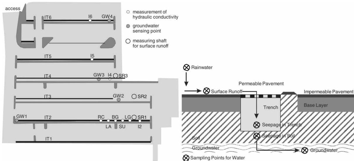
**Figure 1** | Layout of the investigated parking area with measuring equipment and points (left side) and cross section of permeable pavement and infiltration trench (right side).
