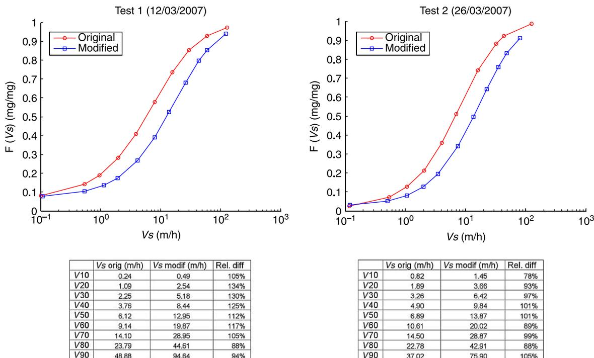
**Figure 2** | Comparison between settling velocity curves obtained from original and modified VICAS protocol for two tests.
