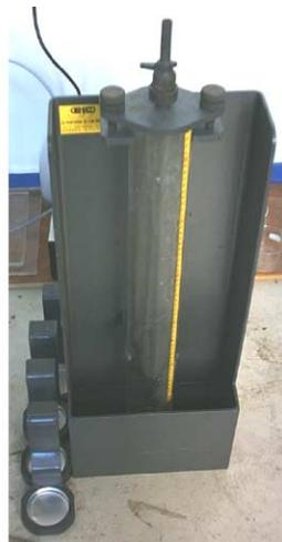
Figure 1 | Scheme (left, adapted from Chebbo *et al.* 2003a) and photo (right, A. Torres) of the VICAS settling column and apparatus.
