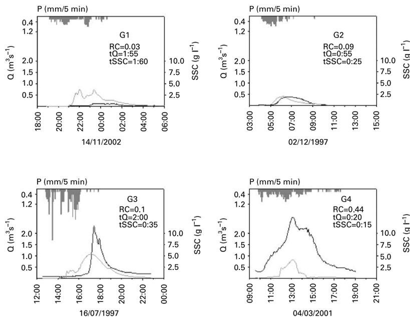
**Figure 3** Hydrographs, sedigraphs and hietographs for each group G1, G2, G3 and G4 (tQ: time lag between the beginning of the rainfall and the beginning of the hydrological response; tSSC: time lag between the beginning of the rainfall and the beginning of sedimentological response)
