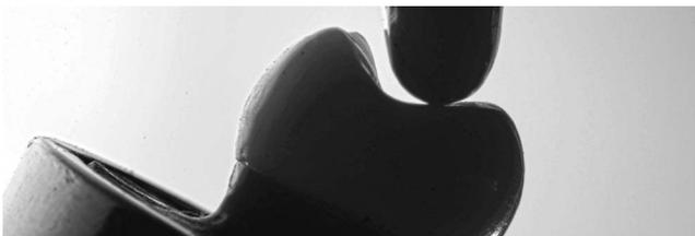
Figure 7. Specimen in load chamber with the loading point equidistant between cuspal tip and central groove.
