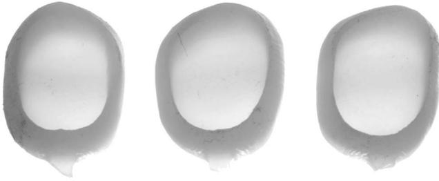
Figure 6. Translucency confirming homogenous material thickness within specimens.
