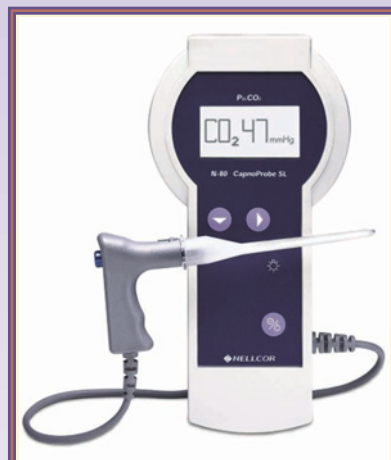
Figure 4 Sublingual capnography probe. The CapnoProbe system (Nellcor, Pleasanton, Calif) uses fiber-optic technology to measure the partial pressure of carbon dioxide in the sublingual tissue ( PslCO_2 ). The carbon dioxide diffuses across the sensor's semipermeable membrane into a fluorescent dye solution. The dye emits light in proportion to the amount of carbon dioxide present. The amount of light emitted is converted into a numerical value.
