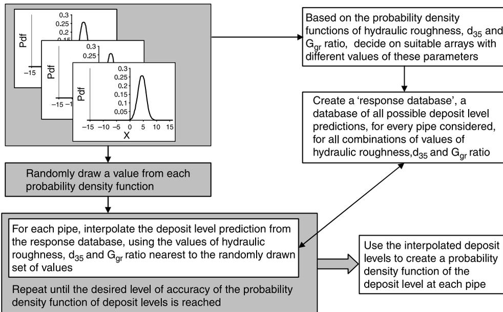
Figure 2 | Schematic illustration of Monte Carlo simulation using a response database.
