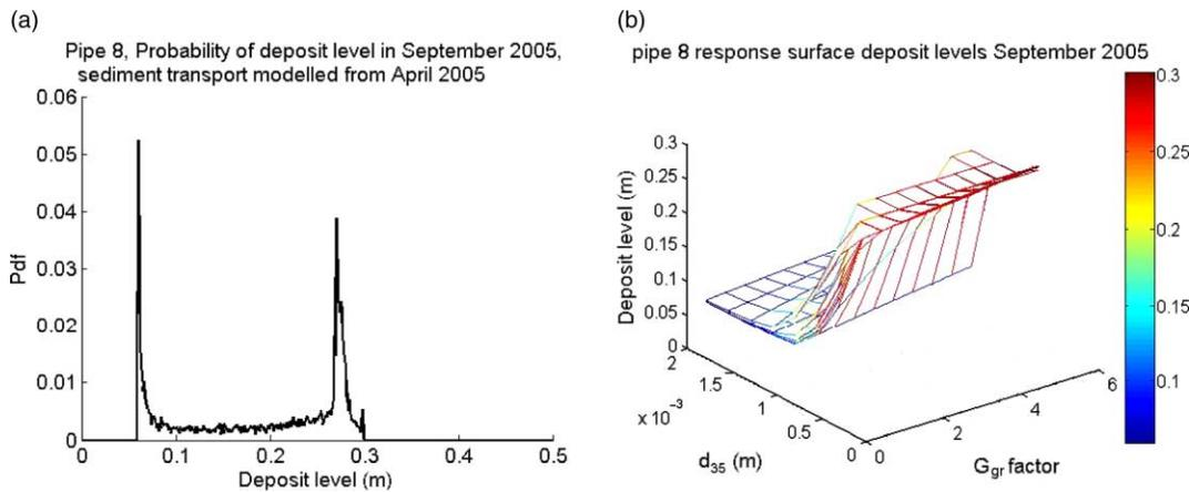
**Figure 4** | Probability density function for deposit depth in pipe 8, and response database for pipe 8, plotted as five 3-D surfaces (one surface for each roughness value). Subscribers to the online version of *Water Science and Technology* can access the colour version of this figure from <http://www.iwapublishing.com/wst>.
