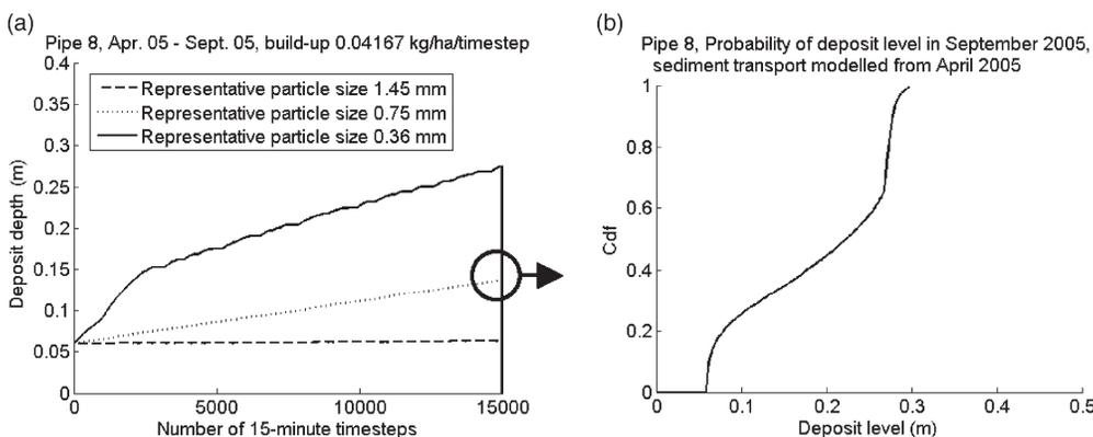
Figure 3 | Comparison between deterministic and probabilistic results of deposit build-up modelling for pipe 8, April 2005 – September 2005.
