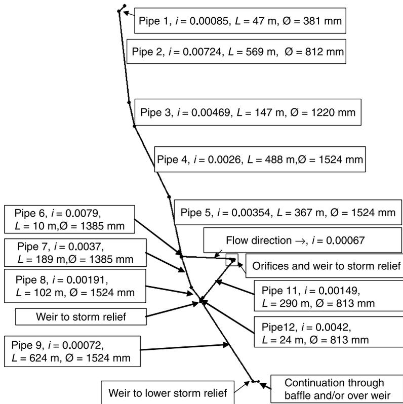
**Figure 1** | Description and location of the pipes coded in the deterministic sediment transport capacity model ( $i$  = invert gradient,  $L$  = length of the pipe,  $\text{Ø}$  = pipe diameter).
