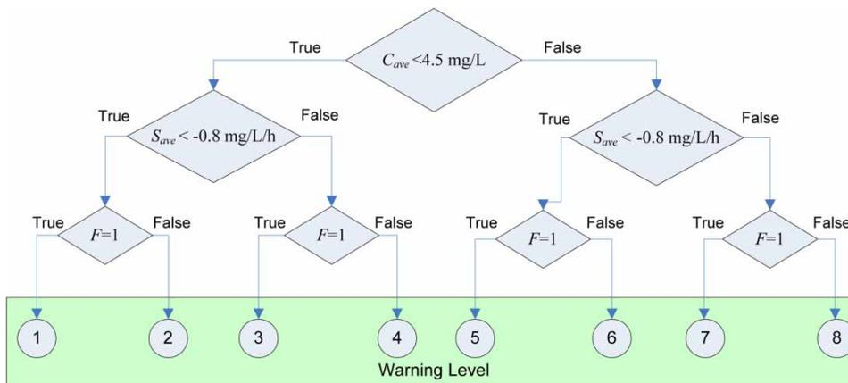
**Figure 6** | Decision tree for the generation of warning levels associated with DO events.  $C_{ave}$  is the average DO concentration,  $S_{ave}$  the average slopes and  $F$  is the continuity in the slope tendency ( $F = 1$  continuous,  $F = 0$  otherwise), all for the last four records.
