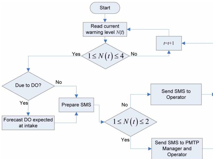
Figure 12 | Flowchart with the rules for SMS delivery.
